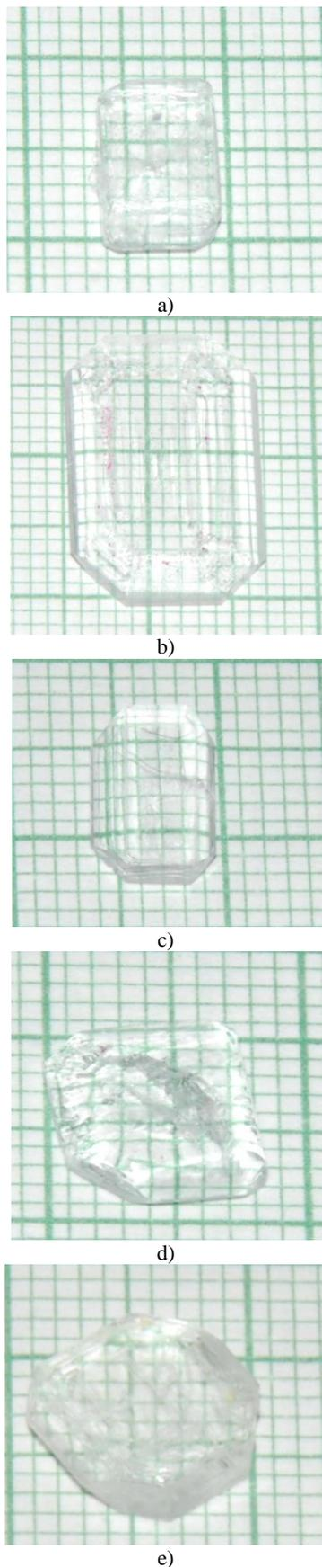
Fig. 1. Photograph of (a) pure (b) cobalt (c) nickel (d) manganese and (e) paranitrophenol doped KDP crystals
