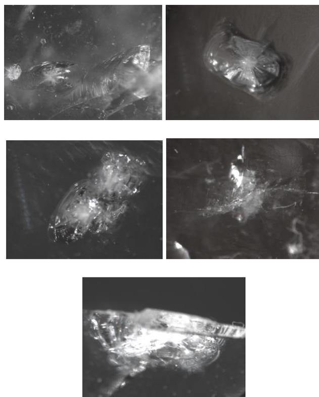
Fig. 3. Laser damage photographs of (a) pure KDP (b) cobalt (c) nickel (d) manganese and (e) paranitrophenol doped KDP crystals
