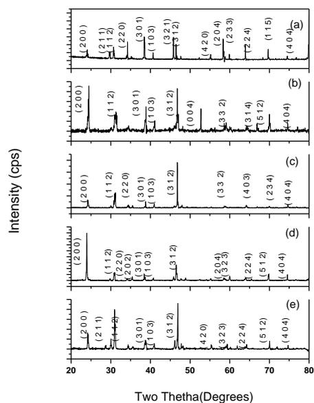
Fig. 2. Powder X-ray diffraction patterns of (a) pure (b) cobalt (c) nickel (d) manganese and (e) paranitrophenol doped KDP crystals
