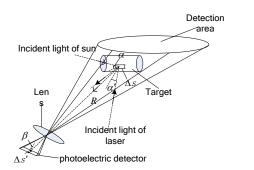
Fig. 2. The space target image principle in photoelectric detection system
