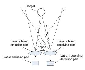
Fig. 1. The detection schematic diagram of laser detection system on space target
