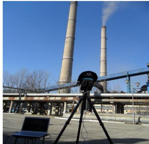
Fig. 3. UV camera placed for the stack monitoring of the Halanga power plant [11].
