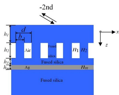
Fig. 1. The schematic diagram of the reflective single-port grating at wavelength of 1550 nm with duty cycle of 0.64 under second Bragg mounting (color online)
