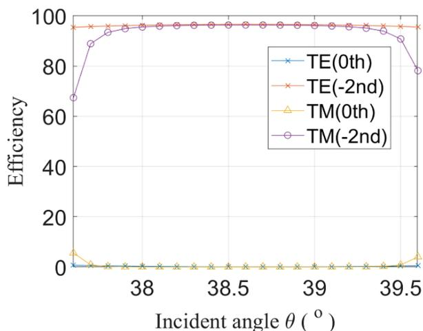
Fig. 5. The diffraction efficiency corresponding to the incident second Bragg angle (color online)
