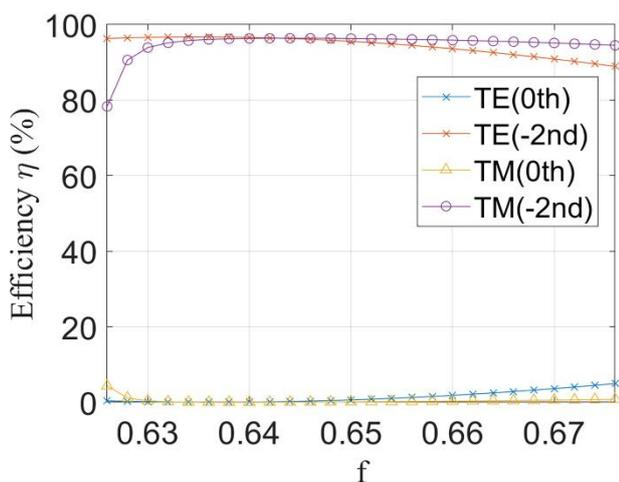
Fig. 6. The diffraction efficiency corresponding to the duty cycle under second Bragg mounting (color online)
