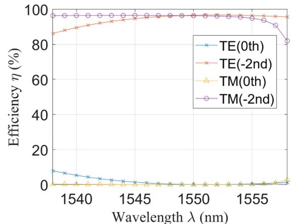
Fig. 4. The efficiency corresponding to the incident wavelength with duty cycle of 0.64 under second Bragg mounting (color online)
