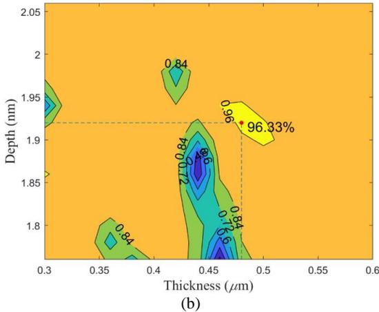
Fig. 2. Reflective efficiencies in the -2nd order versus grating groove depth and the thickness of covering layer for TE and TM polarizations at wavelength of 1550 nm with duty cycle of 0.64 under second Bragg mounting: (a) TE polarization and (b) TM polarization (color online)
