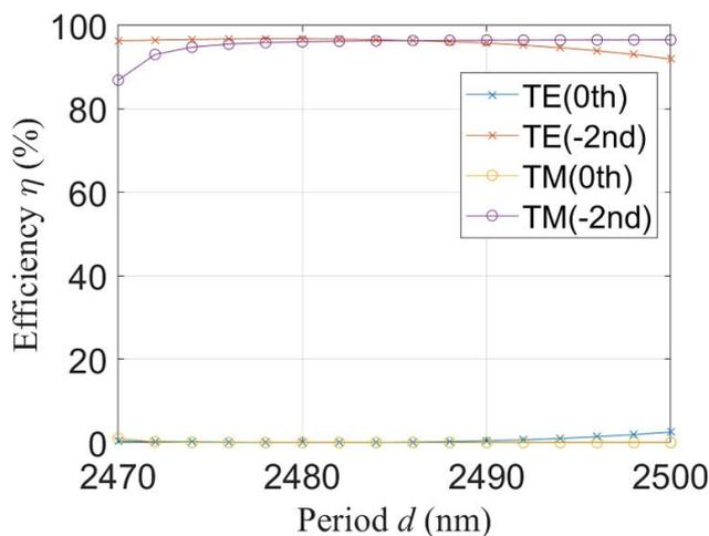
Fig. 7. The efficiency corresponding to the period with duty cycle of 0.64 under second Bragg mounting (color online)
