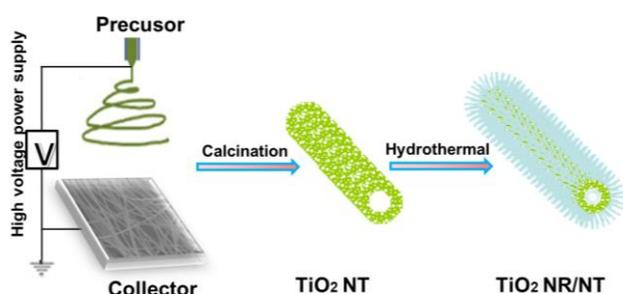
Fig. 1. Schematic representation of TiO<sub>2</sub> NR/NT.
