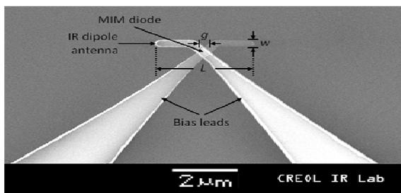
Fig. 1. An electron micrograph of an IR dipole antenna coupled to an MIM diode. From [1].
