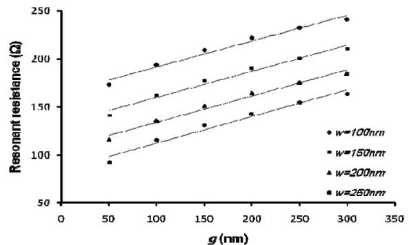
Fig. 5. Antenna resonant input resistance versus antenna feed gap separation ( $g$ ) at various antenna arm widths ( $w$ ).
