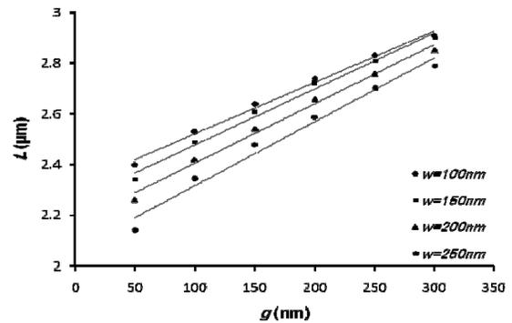
Fig. 4. Antenna resonant length ( $L$ ) versus antenna feed gap separation ( $g$ ) at various antenna arm widths ( $w$ ).
