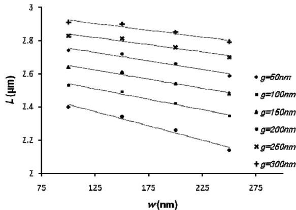
Fig. 2. Antenna resonant length ( $L$ ) versus antenna arm width ( $w$ ) at various antenna feed gap separations ( $g$ ).
