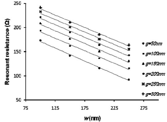
Fig. 3. Antenna resonant input resistance versus antenna arm width ( $w$ ) at various antenna feed gap separations ( $g$ ).
