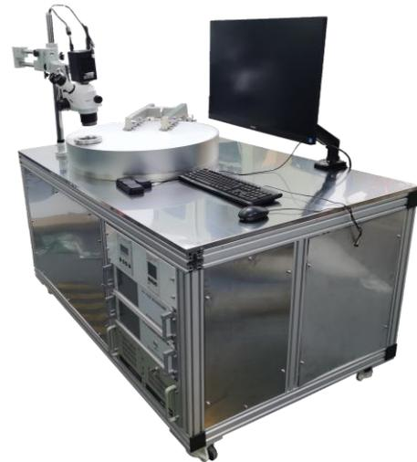
Fig. 3. Picture of rapid and automatic measurement system of phosphor screen performance for image intensifiers
