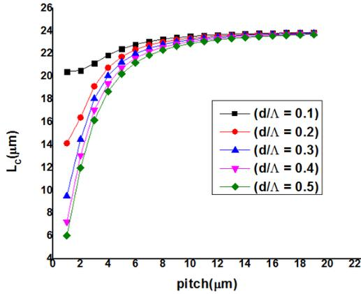
Fig. 5. Coherence length as a function of varying pitch for  $d/\Lambda$  ranging from 0.1 to 0.5
