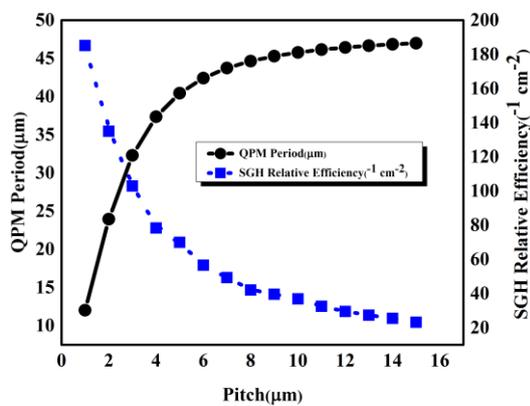
Fig. 9. SGH Relative efficiency (dotted) and QPM period with varying pitch (solid line)
