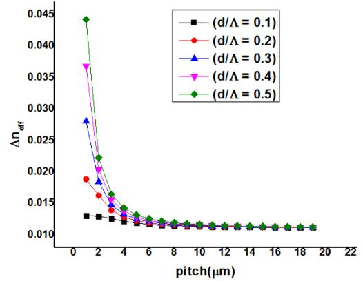
Fig. 3.(b) Variation of effective index difference between fundamental mode and second harmonic mode for various pitch for  $d/\Lambda$  ranging from 0.1 to 0.5
