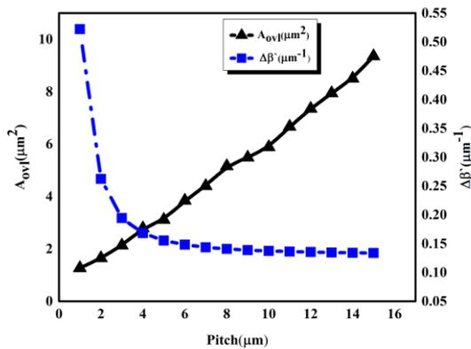
Fig. 8. Relative variation between  $\Delta\beta$  (dotted dash) and  $A_{ovl}$  (solid line) with respect to pitch
