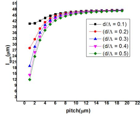
Fig. 6. Quasi-phase matching length as a function of varying pitch for  $d/\Lambda$  ranging from 0.1 to 0.5
