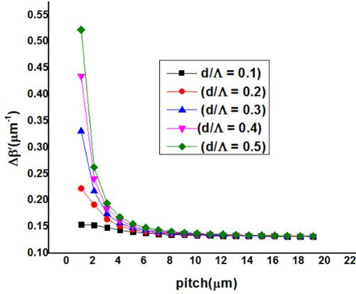
Fig. 4. Variation of wave-vector mismatch for various pitch with for  $d/\Lambda$  ranging from 0.1 to 0.5
