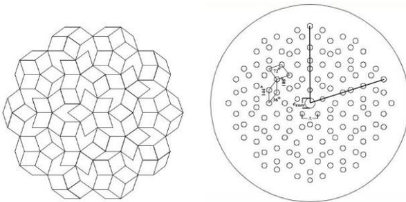
Fig. 1. The geometrical structure of the proposed five-fold symmetric Photonic Quasi crystal fiber
