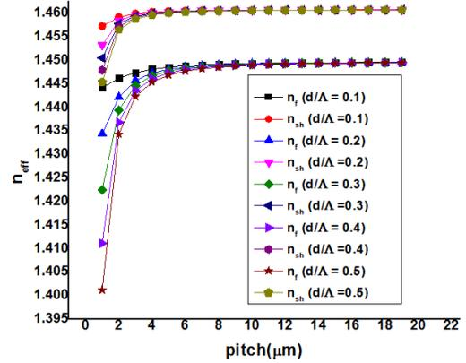
Fig. 3.(a) Change in effective refractive index for fundamental mode and second harmonic mode with reference to increasing pitch for  $d/\Lambda$  ranging from 0.1 to 0.5
