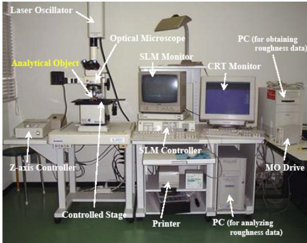
Fig. 2. Whole view of scanning laser microscope system.
