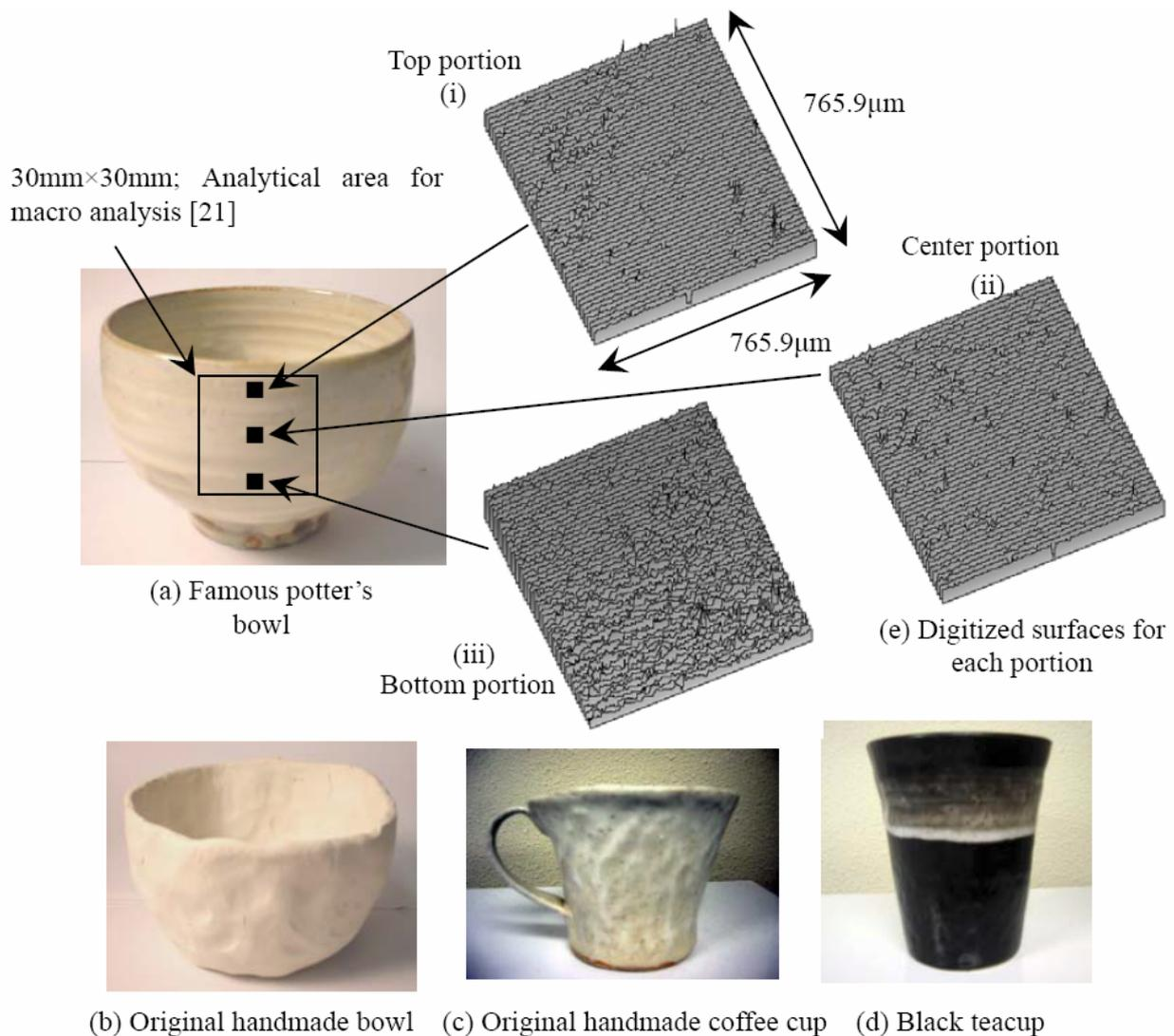
Fig. 1. Photographs of analysis object and digitized surfaces.
