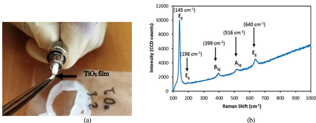
Fig. 1. Characterization of  $\text{TiO}_2$  film (a) Image of fabricated  $\text{TiO}_2$  film (b) Raman spectrum of the fabricated  $\text{TiO}_2$  film
