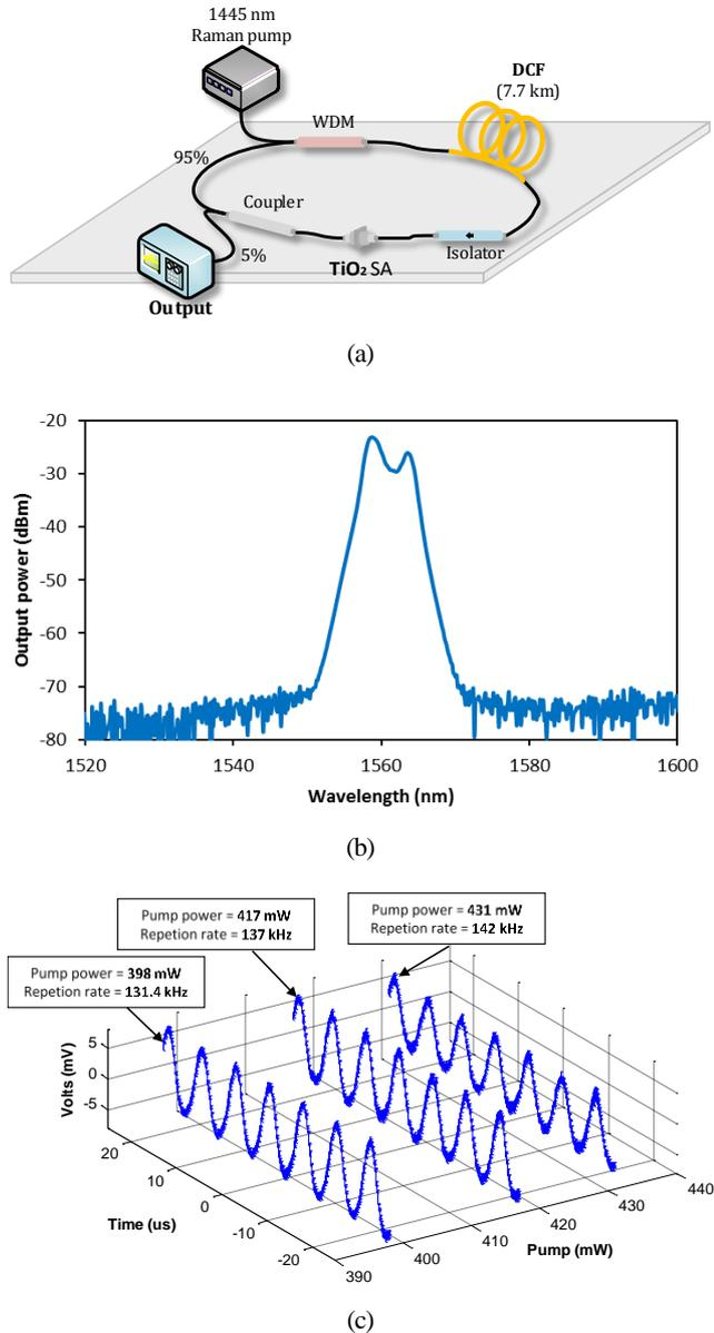
Fig. 2. (a) RFL in a ring cavity configuration. (b) Output spectrum of Q-switched RFL at 431 mW pump power. (c) Typical oscilloscope trace under different pump power between 398 to 431 mW
