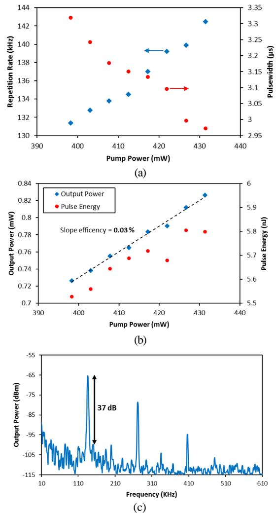
Fig. 3. (a) Repetition rate and pulse width. (b) Output power and pulsed energy. (c) Frequency domain of pulse train at 431 mW pump power
