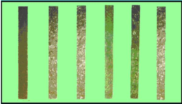
Fig. 1. Glass fiber-reinforced HDPE Polyester for three-point bend tests.
