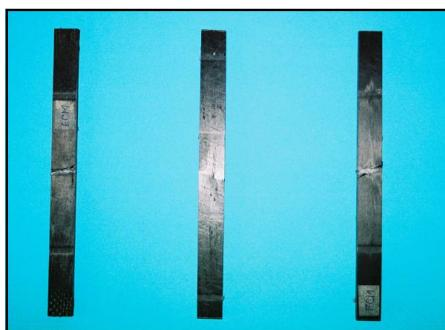
Fig. 9. Carbon fiber-reinforced resin specimens subjected to three-point bend tests.
