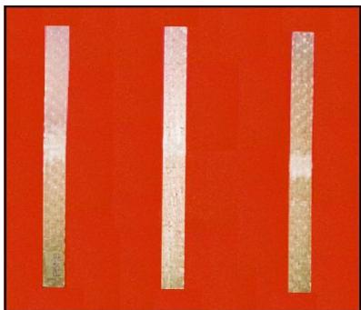
Fig. 7. Specimens of glass fabric-reinforced resin cut on warp direction subjected to three-point bend tests.
