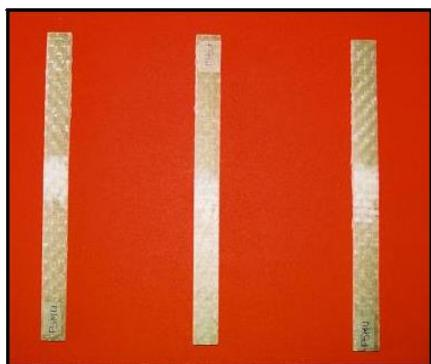
Fig. 8. Broken specimens of glass fabric-reinforced resin cut on weft direction.
