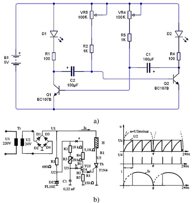
Fig. 2. a) Bi-stabile assemblage for manual adjustment of the ventilation parameters and b) the force power supply
