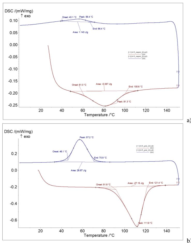
Fig. 4. DSC charts of NiTi wire ( $d=1$  mm) a) initial state and b) after thermal treatment evaluation of the DSC chart recorded at 20°C/min heating rate
