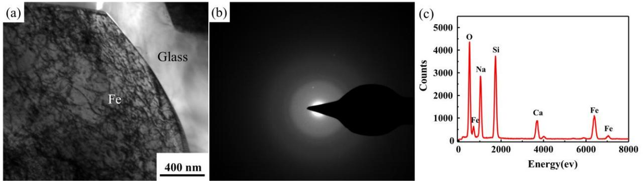
Fig. 4. TEM observation of  $Fe/SiO_2-Na_2O-CaO$  composites. (a) interface, (b) electron diffraction pattern and (c) EDS analysis of amorphous  $SiO_2-Na_2O-CaO$ .
