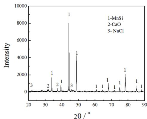
Fig. 2. XRD pattern of sintered  $\text{MnO}_2\text{-SiO}_2$  pellets after electrolyzing (Ball-milled for 3 h, compacted at 20 MPa, sintered at  $850^\circ\text{C}$  for 6 h, and electrolyzed in molten  $\text{CaCl}_2\text{-NaCl}$  at  $850^\circ\text{C}$  for 19 h under 3.10 V).
