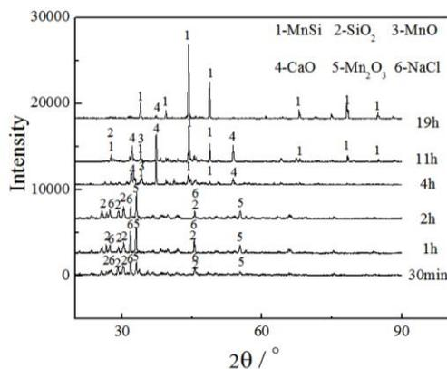
Fig. 4. XRD pattern of sintered  $\text{MnO}_2\text{-SiO}_2$  pellets after electrolyzing at different time (30 min, 1 h, 2 h, 4 h, 11 h, and 19 h) (Ball-milled for 3 h, compacted at 20MPa, sintered at  $850^\circ\text{C}$  for 6 h, and electrolyzed in molten  $\text{CaCl}_2\text{-NaCl}$  at  $850^\circ\text{C}$  for 13 h under 3.10 V).
