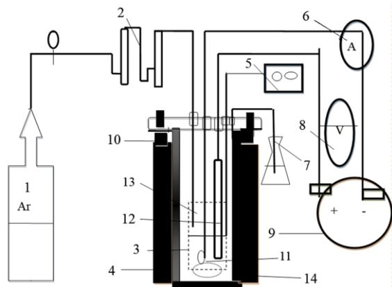
Fig. 1. Sketch map of electrolysis equipment (1-Ar cylinder; 2-spray drying tower; 3-alumina crucible; 4-stainless steel tube reactor; 5-thermocouple; 6-ammeter; 7-tail gas absorption bottle; 8-ammeter; 9-DC voltage stabilizer; 10-cooling water; 11- $\text{SiO}_2\text{-MnO}_2$  pellet; 12-graphite rod; 13- $\text{CaCl}_2\text{-NaCl}$  melts; 14-heating furnace).
