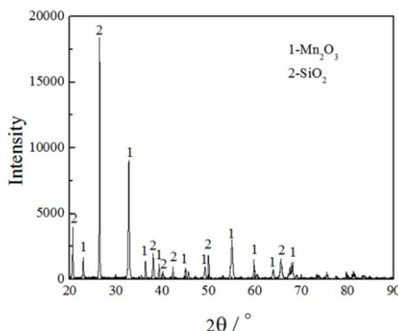
Fig. 3. XRD pattern of  $\text{MnO}_2\text{-SiO}_2$  pellets sintered at  $850^\circ\text{C}$  for 6 h.
