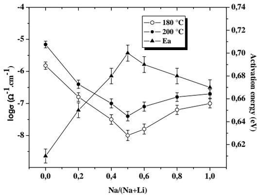
Fig. 3. Plots of conductivity and activation energy versus composition along the glass system  $0.5[x(2\text{NaF})-(1-x)\text{Li}_2\text{O}]-0.5[0.25(\text{WO}_3)_2-0.75\text{P}_2\text{O}_5]$ . Line is drawn as guide to the eye.
