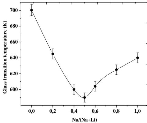
Fig. 4. Composition change of the glass transition temperature for the glass system  $0.5[x(2\text{NaF})-(1-x)\text{Li}_2\text{O}]-0.5[0.25(\text{WO}_3)_2-0.75\text{P}_2\text{O}_5]$ . Line is drawn as guide to the eye.
