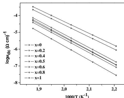
Fig. 2. Thermal variation of the dc conductivity along the system  $0.5 [x(2\text{NaF})-(1-x)\text{Li}_2\text{O}]-0.5 [0.25(\text{WO}_3)_2-0.75\text{P}_2\text{O}_5]$ .
