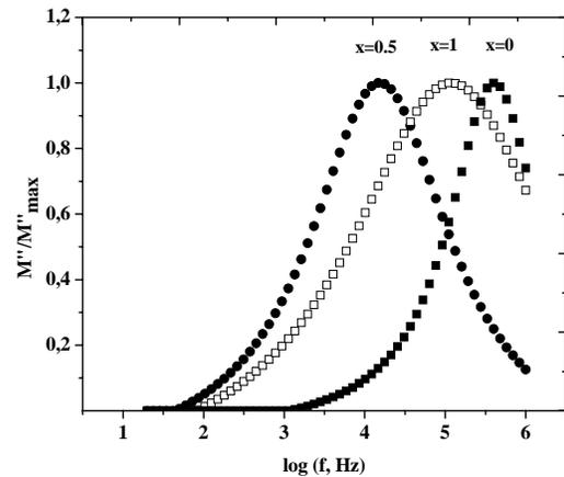
Fig. 6. Frequency dependence of the imaginary part of the normalized dielectric modulus  $M''/M''_{\text{max}}$  for the two single Li and Na and mixed Li-Na ( $x = 0.5$ ) glasses.
