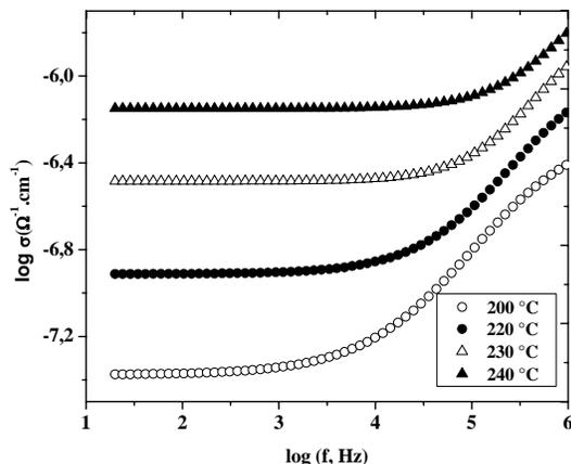
Fig. 5. Typical example of the ac conductivity of the glass composition  $0.5[x(2\text{NaF})-(1-x)\text{Li}_2\text{O}]-0.5[0.25(\text{WO}_3)_2-0.75\text{P}_2\text{O}_5]$  ( $x = 0.6$ ).
