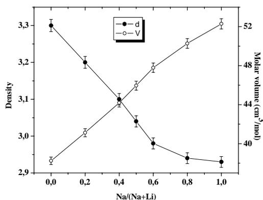
Fig. 1. Plots of density and molar volume versus the molar ratio  $\text{Na}/(\text{Na}+\text{Li})$  along the system  $0.5[x(2\text{NaF})-(1-x)\text{Li}_2\text{O}]-0.5[0.25(\text{WO}_3)_2-0.75\text{P}_2\text{O}_5]$ .
