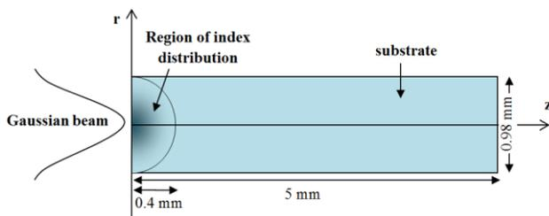
Fig. 1. Schematic illustration of a GRIN PML and its dimensions
