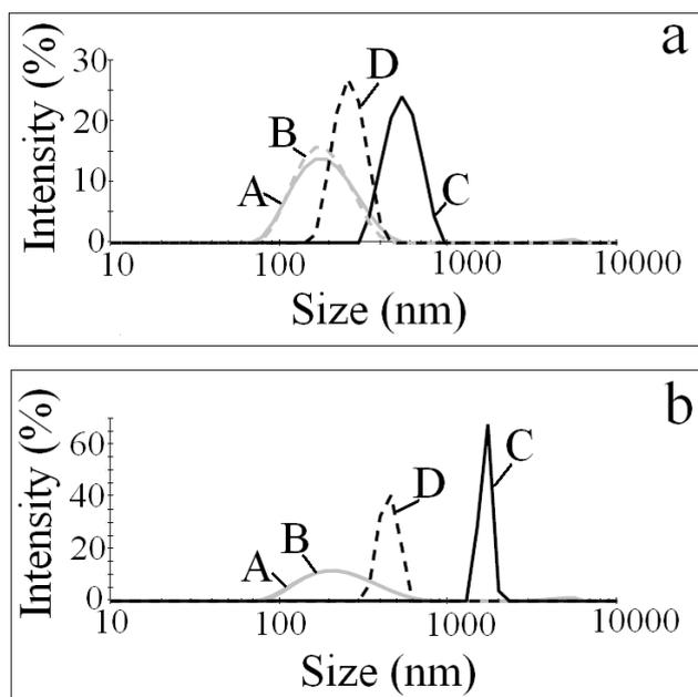
Fig. 2. Distribution by intensity for: a) PSSt latexes; b) PMMA latexes (A-blank latex 20°C; B-blank latex 50°C; C-colored latex 20°C; D-colored latex 50°C).
