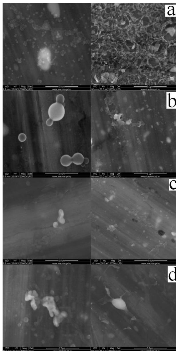
Fig. 3. SEM images obtained for the final systems with styrene (a), butylacrylate (b), vinyl acetate (c) and acrylonitrile (d), for the neat samples (left) and those obtained in the presence of the colored complex (right).
