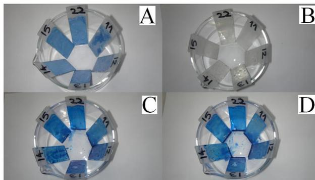
Fig. 1. Thermochromic systems (11 dye-PSt; 12 dye-PBuA; 13 dye-PMMA; 14 dye-PVAc; 15 dye-PACN; 22 dye-P(St-BuA)) deposited on glass tiles at: A-room temperature; B-60 °C; C-room temperature, after 1 h at 60 °C; D-room temperature, after 2 h at 60 °C.
