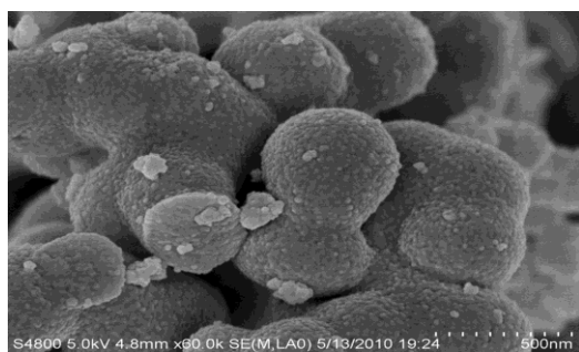
Fig. 4. SEM of powder pattern of TiO 2 -PAN particle.
