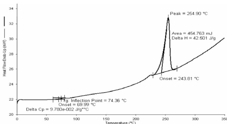
Fig. 1. DSC spectrum of PET substrate.
