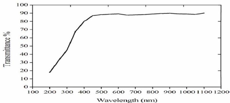
Fig. 6. Optical transmission of PET substrate.
