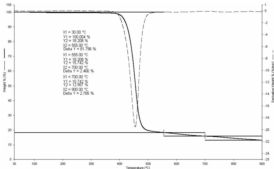
Fig. 2. The thermogravimetric data of PET compounds.
