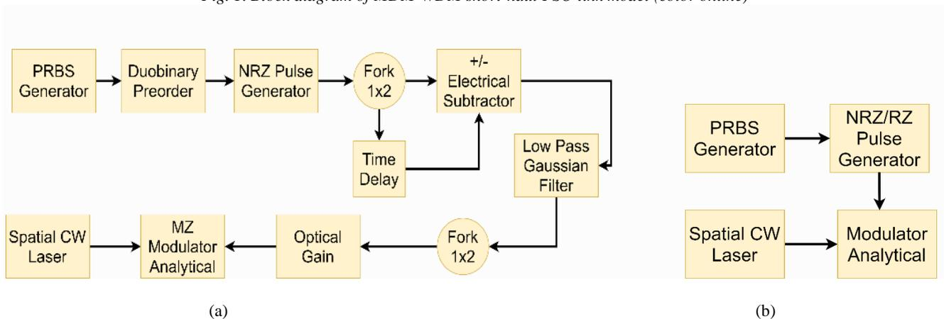
Fig. 2. Block diagram of transmitter, (a): AMI transmitter, (b): NRZ/RZ transmitter
