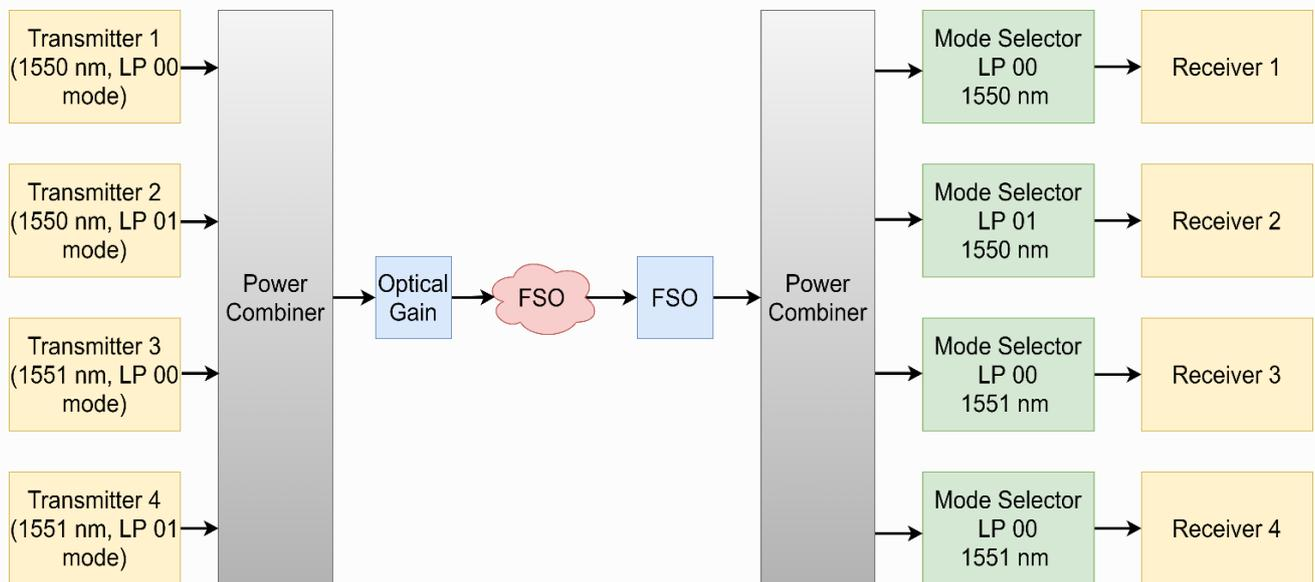
Fig. 1. Block diagram of MDM-WDM short-haul FSO link model (color online)
