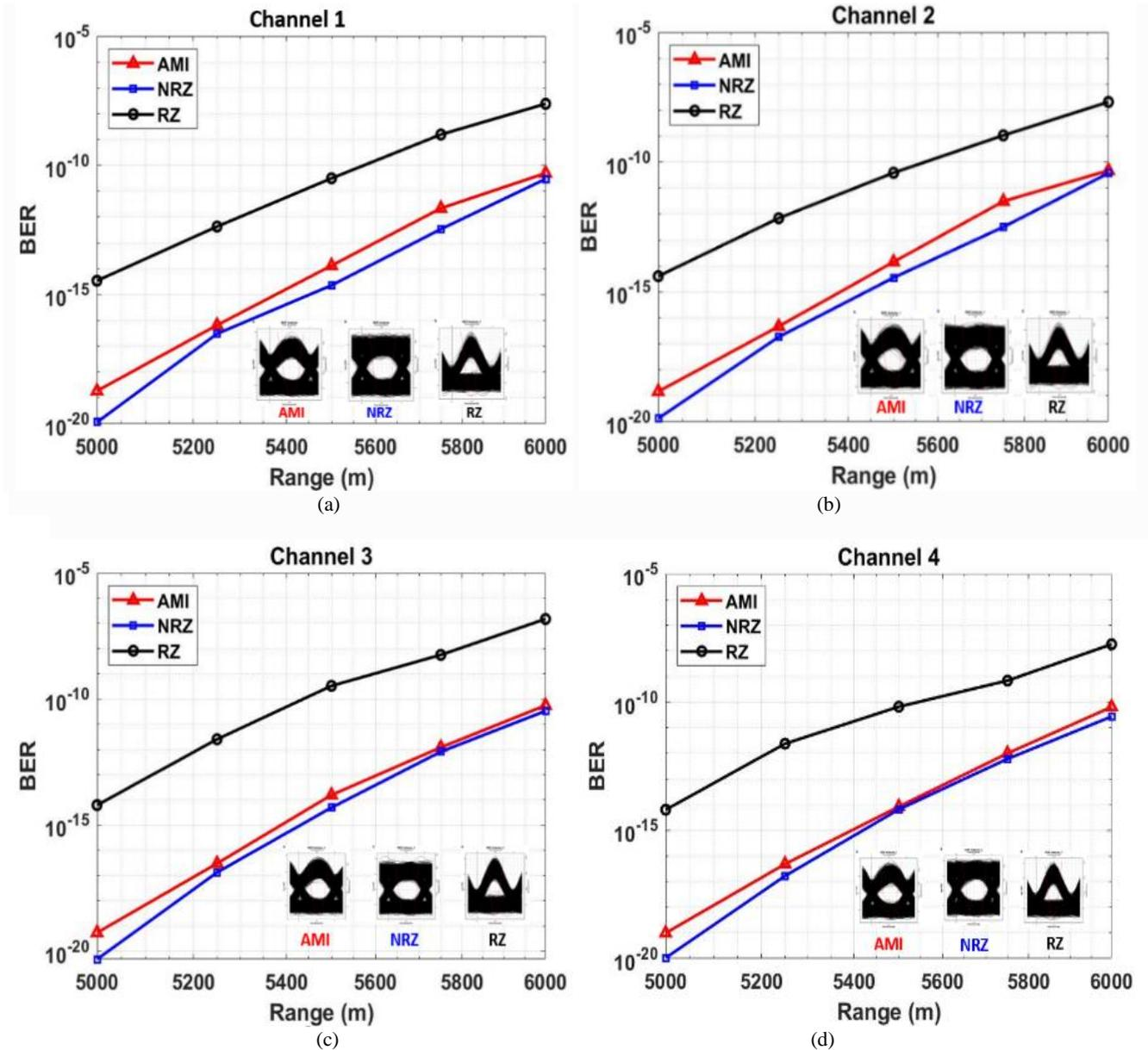
Fig. 5. BER versus range comparing AMI, NRZ and RZ encoding techniques for: (a) channel 1, (b) channel 2, (c) channel 3 and (d) channel 4 (color online)
