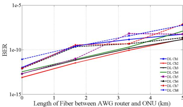
Fig. 7. Downlink BER versus fiber length between AWG router and ONU.
