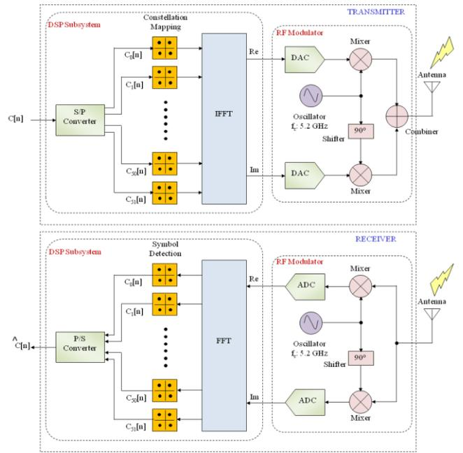
Fig. 5. OFDM based IEEE 802.11a transmitting and receiving systems.
