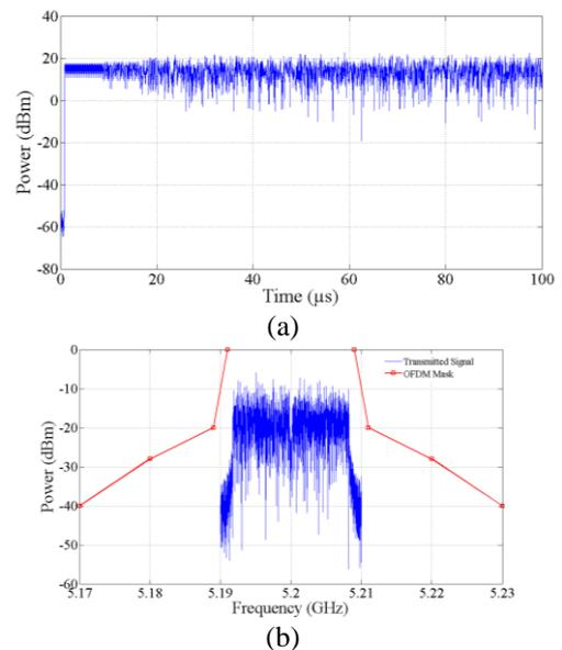
Fig. 9. The transmitted RF power signal at AP (a) in time domain (b) in frequency domain.
