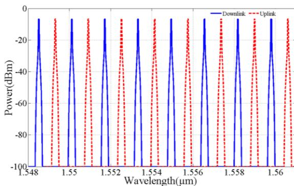
Fig. 4. Allocated wavelengths of the downlink/uplink channels for the optical backhaul.
