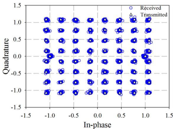
Fig. 10. The constellations of the transmitted and received RF power signal.
