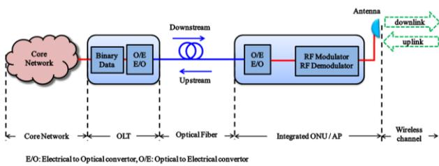
Fig. 2. Integrated optical-wireless system architecture.
