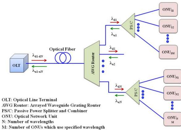
Fig. 3. Optical backhaul architecture.
