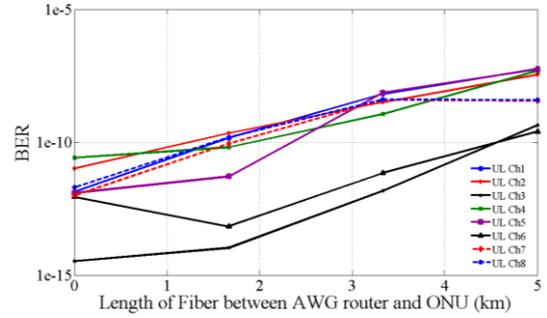
Fig. 8. Uplink BER versus fiber length between AWG router and ONU.
