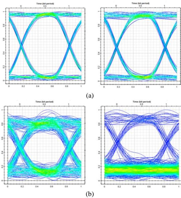
Fig. 6. Eye diagrams of the optical backhaul measured at ONU (left) and OLT (right) with split ratio (a) 1/8 (b) 1/32.
