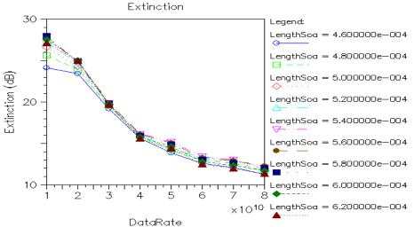
Fig. 13. Extinction vs. data rate vs. Length of SOA
