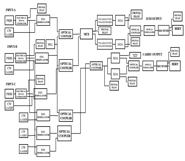
Fig. 1(a). The Full Adder Design
