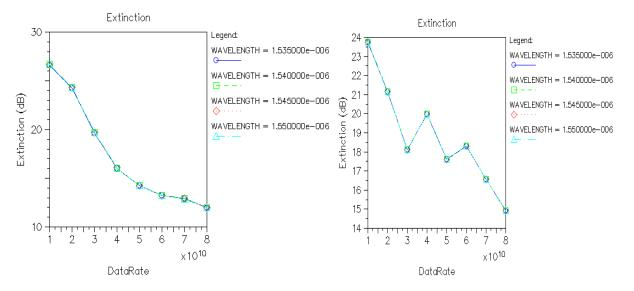
Fig. 14. Full Adder Extinction vs. data rate wavelength (a) Sum (b) Carry
