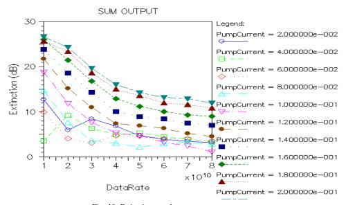
Fig. 10. Extinction vs. data rate vs. pump current
