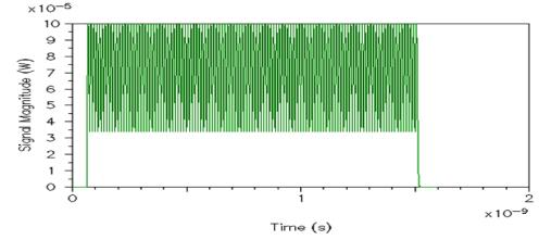
Fig. 1(b). Mode locked laser output
