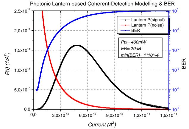
Fig. 4. Minimum BER calculation
