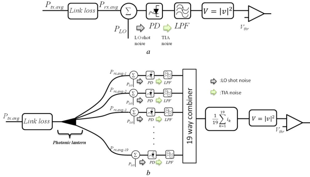
Fig. 2. Model of detection system for single-mode fiber (a), and photonic lantern (b) based coherent systems
