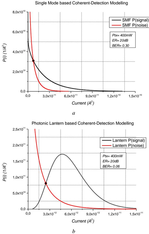
Fig. 3. Probability density functions for (a) single-mode based receiver (b) photonic lantern based receiver
