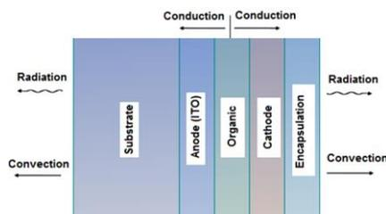
Fig. 1. The OLED heat transfer mechanism
