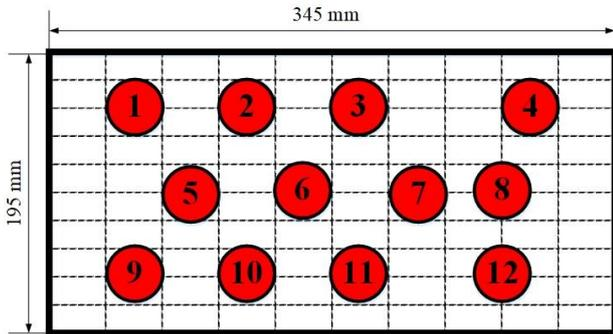
Fig. 3. Placement of the thermocouples
