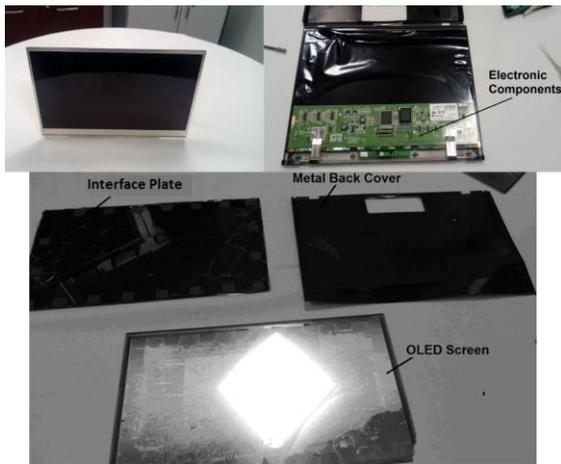
Fig. 2. OLED device components
