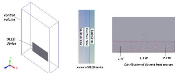
Fig. 6. Simulation model of OLED device
