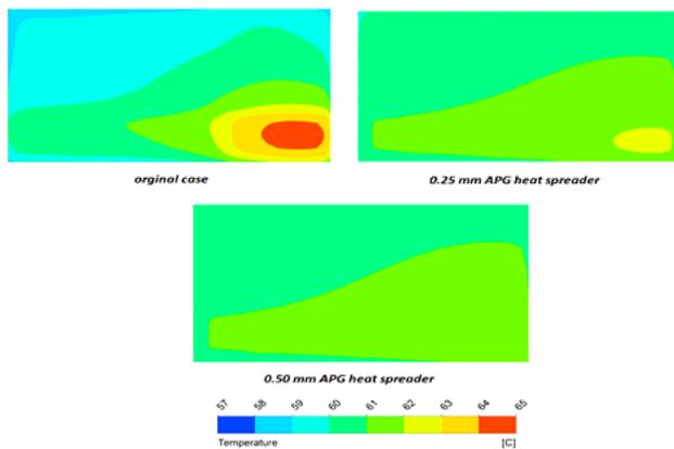
Fig. 10. Temperature distributions for APG heat spreader at different thickness
