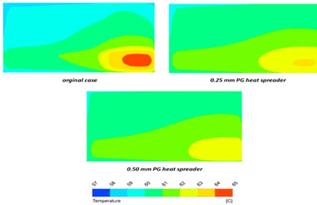
Fig. 9. Temperature distributions for PG heat spreader at different thickness
