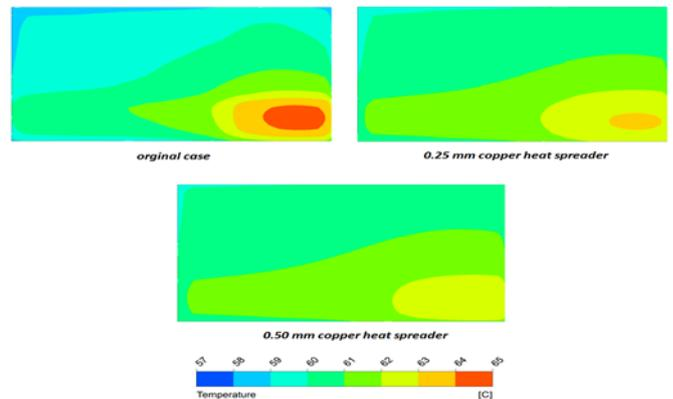
Fig. 8. Temperature distributions for copper heat spreader at different thickness
