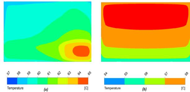
Fig. 7. Simulation results of the temperature distribution on the OLED display screen
