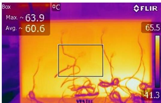
Fig. 4. OLED Thermal camera temperature distributions
