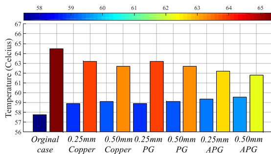
Fig. 11. Maximum and minimum temperatures on the OLED display
