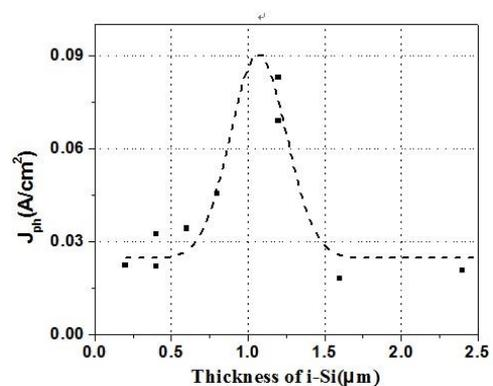
Fig. 4. The  $J_{ph}$  of the fabricated  $p^+$ -Si/i-Si/n-SiC heterojunction photodiode with different i-Si thickness under visible illumination.
