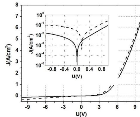
Fig. 3. The electrical and photoelectrical characteristics of the fabricated  $p^+$ -Si/i-Si/n<sup>+</sup>-SiC heterojunction photodiode.
