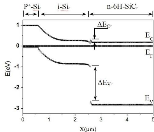
Fig. 1. Energy-band diagram for the  $p^+$ -Si/i-Si/n-SiC heterostructure in equilibrium.
