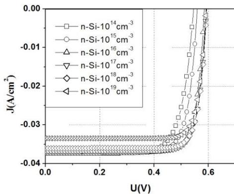
Fig. 2. Simulated photoelectrical characteristics of the  $p^+$ -Si/i-Si/n-SiC photodiode under visible illumination with different doping concentrations of i-Si layer.
