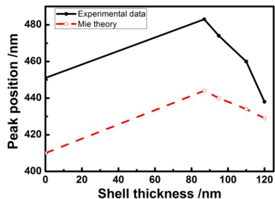
Fig. 5. Variation in the position of the plasmon band of 50 nm Ag particles with silica thickness: (solid circles) experimental data; (open circles) calculated positions.
