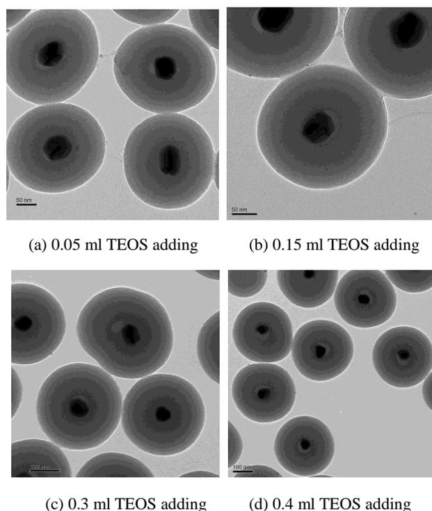
Fig. 2. TEM images of Ag@SiO<sub>2</sub> core-shell particles.
