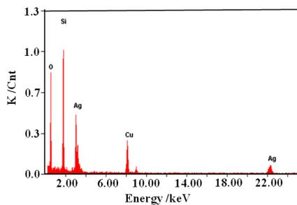
Fig. 3. EDS spectrum of Ag@SiO<sub>2</sub> core-shell particles.
