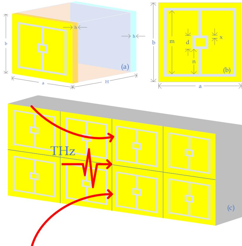
Fig. 3. The structure of metamaterial unit device (a) unit cell structure; (b) unit cell front structure; (c) metamaterial absorber schematic (color online)
