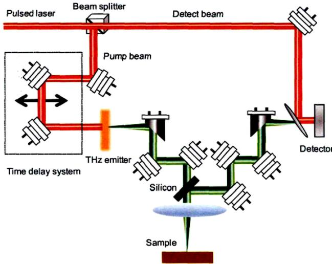
Fig. 1. Reflection detection mode of terahertz time domain spectroscopy system (color online)
