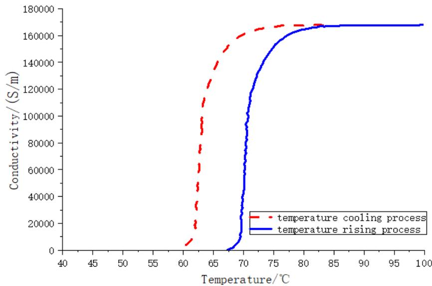
Fig. 2. Relationship between conductivity and temperature of  $\text{VO}_2$  film (temperature rising process  $T_0 = 68^\circ\text{C}$ , cooling process  $T_0 = 62^\circ\text{C}$ ) (color online)
