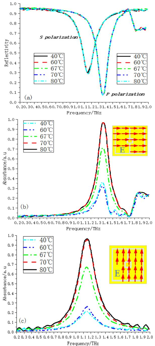
Fig. 5. Reflection and absorption lines of two polarization incident THz waves at different temperatures. (a) absorption line; (b) absorption line of P polarization; (c) absorption line of S polarization (color online)
