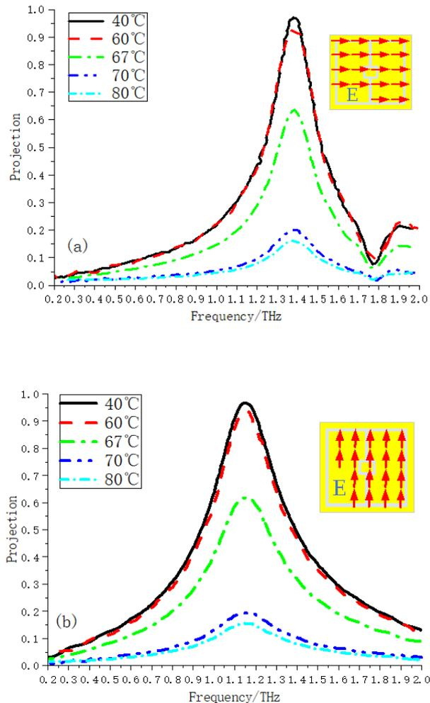
Fig. 4. Transmission line of two polarization incident THz waves at different temperatures (a) P polarization; (b) S polarization (color online)
