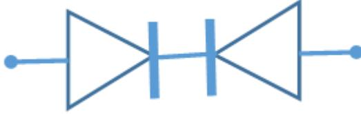
Fig. 8. Equivalent circuit of two semiconductor diodes connected in opposite
