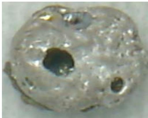
Fig. 2. Sample of  $\text{CuGaS}_2$  Showing a poor morphology.
