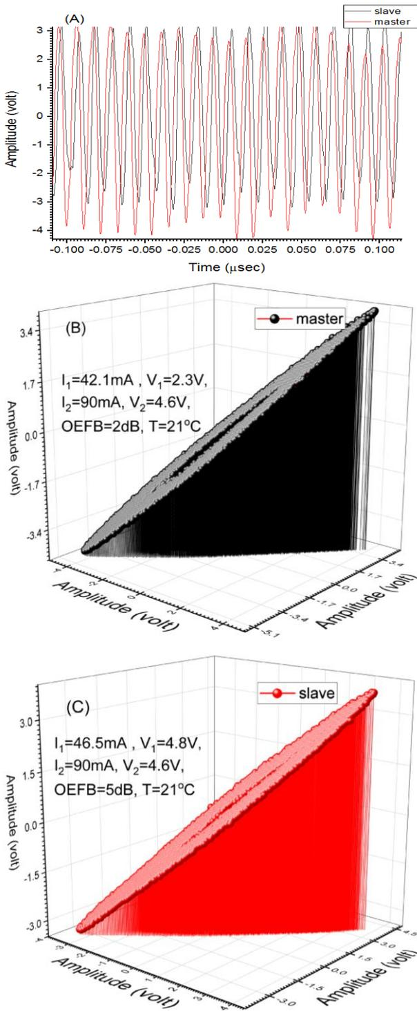
Fig. 5. Measured M-S dynamics in transmittance unite. "(A)" Time series, "(B)" and "(C)" M and S chaotic attractors, respectively (color online)
