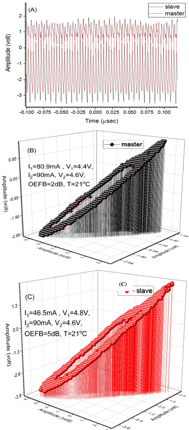
Fig. 12. Results for M-S dynamics in transmittance unite. "(A)" time series, "(B)", and "(C)" are two signals periodic attractors for M and S, respectively (color online)
