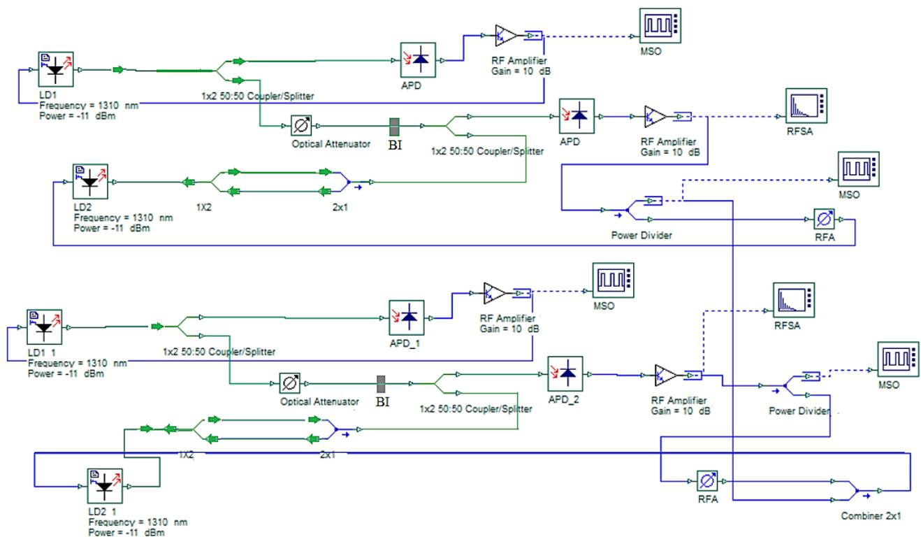
Fig. 1. Experimental set-up for closed-loop chaotic synchronization based on HFBI technique, abbreviations are reported during the text (color online)
