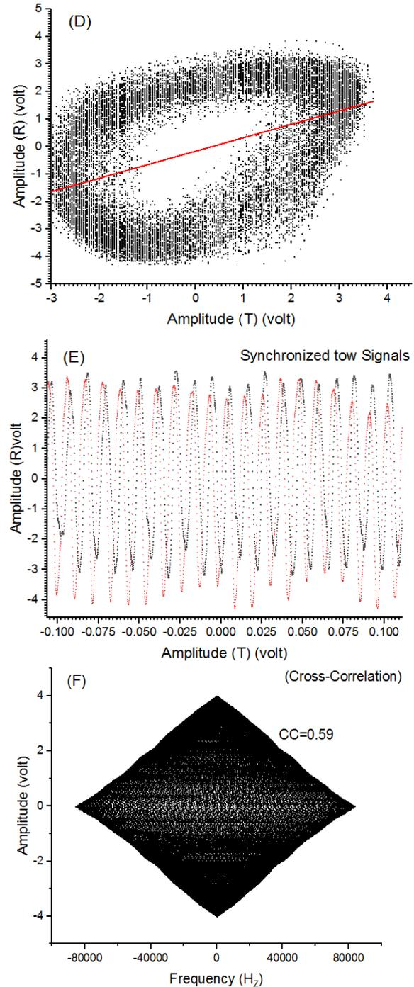
Fig. 6. Calculations and examination for M-S Cross-Correlation for data achieved from Fig. 5. "(D)" synchronization diagram, "(E)" Synchronized two signals, and "(F)" Cross-Correlation (color online)
