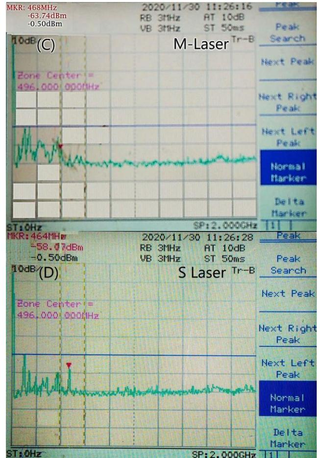
Fig. 14. Fourier (RF) spectra for M and S lasers signal from observations given in Fig. 12, "(C)" M laser, "(D)" S laser (color online)
