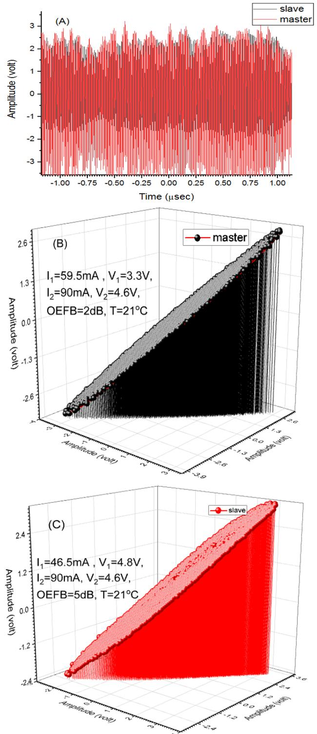
Fig. 9. Measured Master - Slave (M-S) dynamics in transmittance unite. "(A)" time series, "(B)" and "(C)" their chaotic attractors (color online)
