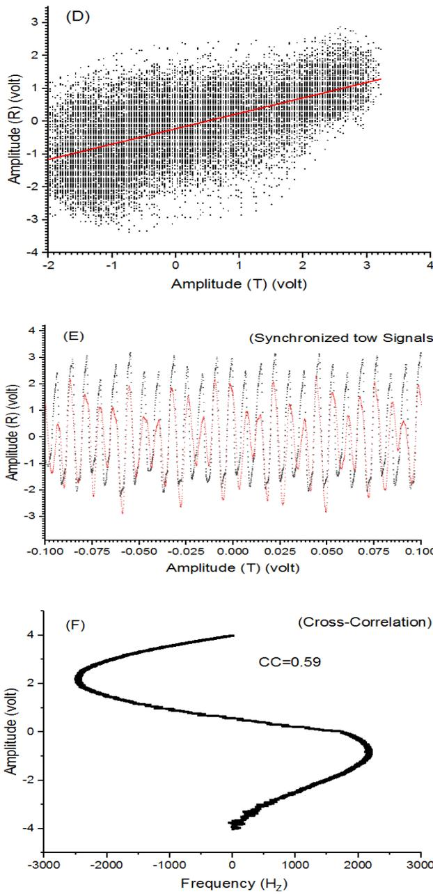
Fig. 8. Calculations and examination for M-S Cross-Correlation for data achieved from Fig. 7. "(D)" synchronization diagram, "(E)" Synchronized two signals, and "(F)" Cross-Correlation (color online)
