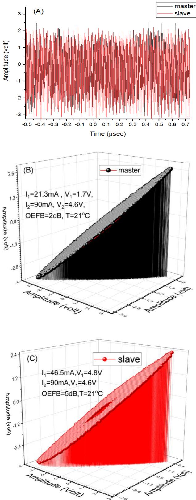
Fig. 2. Measured Master - Slave (M-S) resulted chaotic dynamics in transmittance unite. "(A)" time series, "(B)" and "(C)" their chaotic attractors (color online)
