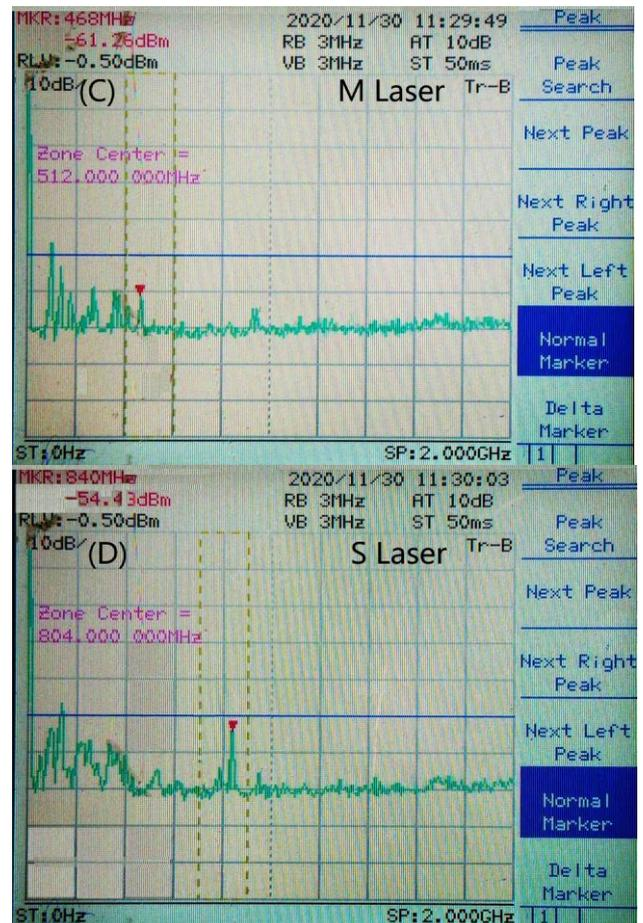
Fig. 11. Fourier (RF) spectra for M and S lasers signal from observations given in Fig. 9, "(C)" M laser, "(D)" S laser (color online)
