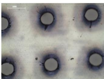
Fig. 15. The same hole matrices used this time for drilling holes in PET.
