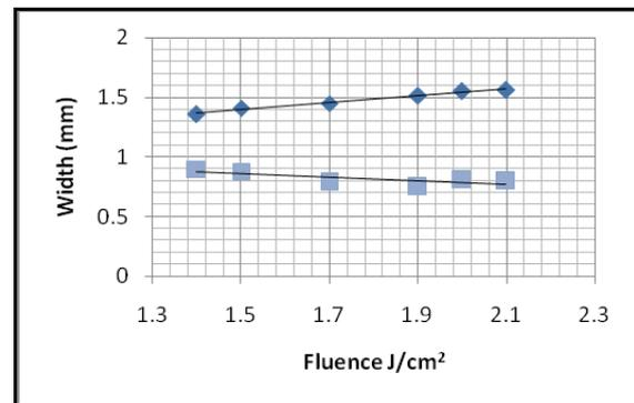
Fig. 12. Evolution of width in the top and bottom side channels as a function of laser's fluence.
