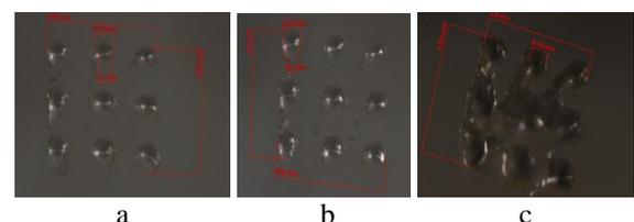
Fig. 7. The effect of laser energy density and repetition rate on the PMMA for 100 pulses, at a fluence of 1.5 J/cm<sup>2</sup> and 3 frequencies a)1Hz b) 5Hz c) 10Hz .
