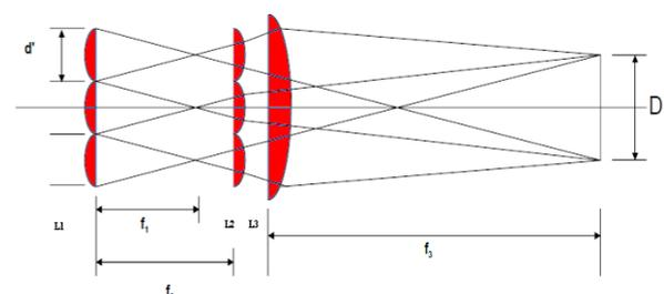
Fig. 2. The homogenizer principle.
