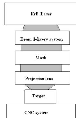
Fig. 1. The experimental block diagram.
