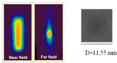
Fig. 4. Intensity distribution before (a) and after (b) homogenization.
