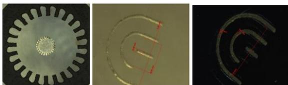
Fig. 13. A wheel structure made in PMMA and ~ 100  $\mu\text{m}$  channel structure made in PMMA and Si.
