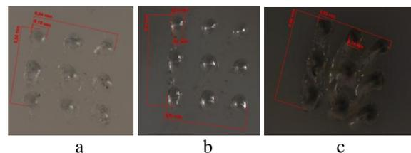
Fig. 6. The effect of laser energy density and repetition rate on the PMMA. We used 100 pulses, a fluence of  $0.8$  J/cm<sup>2</sup> and 3 frequencies a) 1Hz b) 7Hz c) 15Hz .
