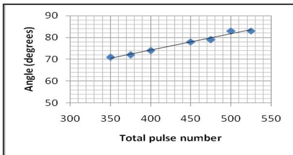
Fig. 10. Influence of the total number of pulses on the angle between hole's wall and entrance surface.
