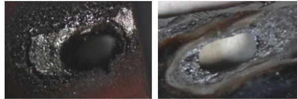
Fig. 5. Non-uniform laser spot shape obtained in Si and ferromagnetic material by using a single plane-convex lens.
