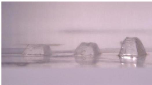
Fig. 9. Some results of testing the influence of number of pulses over the hole's wall for 300,400 and 550 pulses. The more the pulses the closer to 90 deg the angle between the surface and the hole wall.
