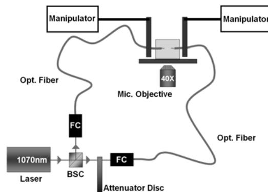
Fig.3. The schematics of the optical tweezers setup. The beam of the 1043nm laser was divided in to two by a beam splitter cube (BSC). The two beams than were coupled (FC) in to the optical fibers while the two other ends were hold by two independent manipulator in the test volume which took place on the motorized stage and was observed by the objective of the inverted microscope from the bottom.
