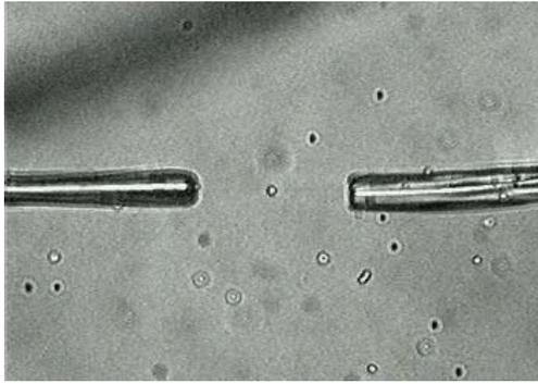
Fig. 4. An image of the tweezers trapping a bead.
