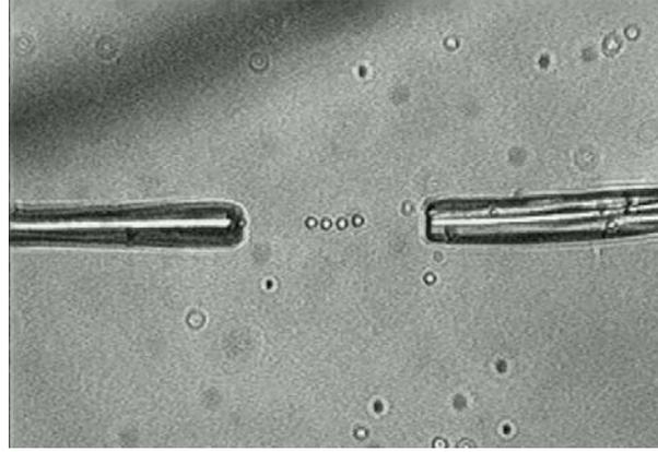
Fig. 5. Optical binding observed. The optical forces hold four beads in line between the tips.
