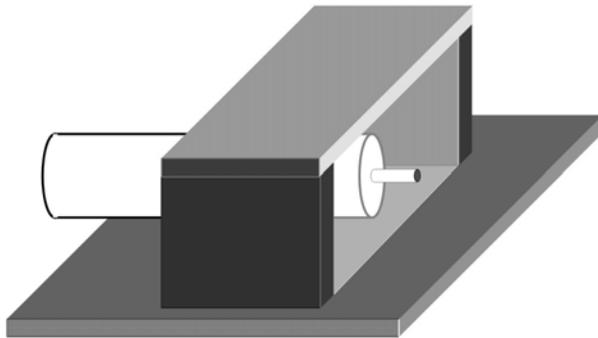
Fig.1. Scheme of the chamber to grow the tip by photopolymerisation. The left and right sides of the brick shaped chamber are open, and the resin is held in place by surface tension.
