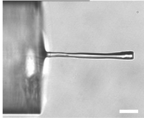
Fig. 2. Image of a typical tip grown at the end of the optical fiber. One can notice the flat end. The white bar represents 20 micrometers.
