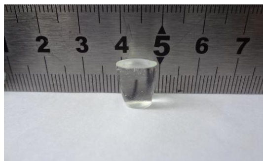
Fig. 2. The sample rod of \text{Tm}^{3+} -doped silica rod fabricated by NCVD.
