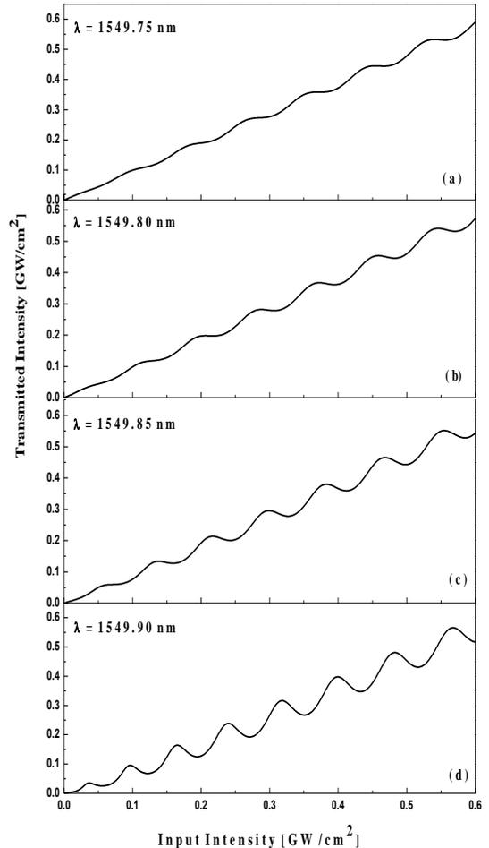
Fig. 1. Transmitted vs. incident intensity for a nonlinear fiber Bragg grating for different values of detuning wavelengths.
