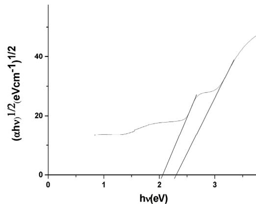
Fig. 11. Indirect allowed transition energy gap of PANI(EB) cast from NMP.
