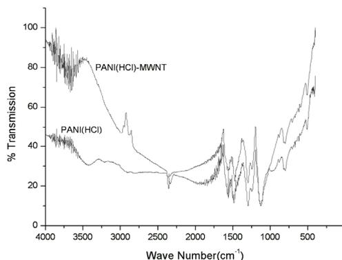
Fig. 2. FTIR spectra of PANI (HCl) and PANI (HCl)-MWNT (1:0.5) composite.
