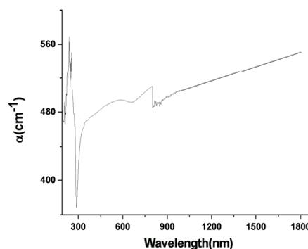
Fig. 8. Optical absorption spectrum of PANI(HCl)-MWNT(1:0.5) composite.
