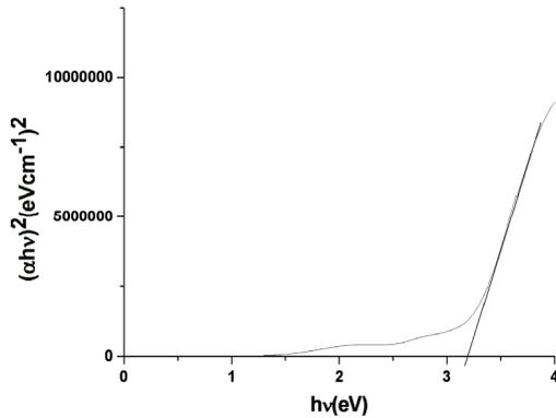
Fig. 9. Direct allowed transition energy gap of PANI(EB) cast from NMP.
