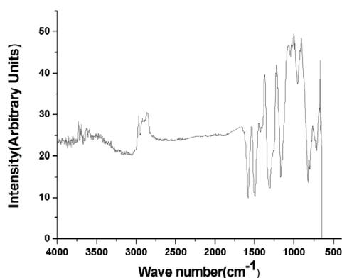
Fig. 1. FTIR spectrum of PANI (EB).
