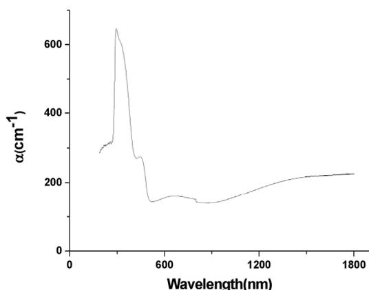
Fig. 5. Optical absorption spectrum of PANI (EB) cast from NMP.
