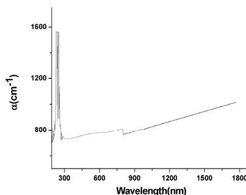
Fig. 7. Optical absorption spectrum of PANI(HCl).
