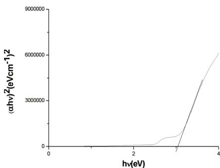
Fig. 10. Direct allowed transition energy gap of PANI(EB) cast from m-cresol.
