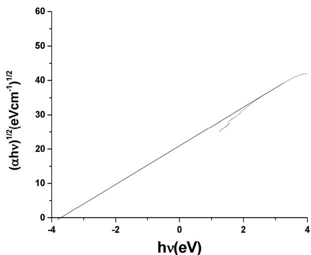
Fig. 14. Indirect allowed transition energy gap of PANI(HCl).
