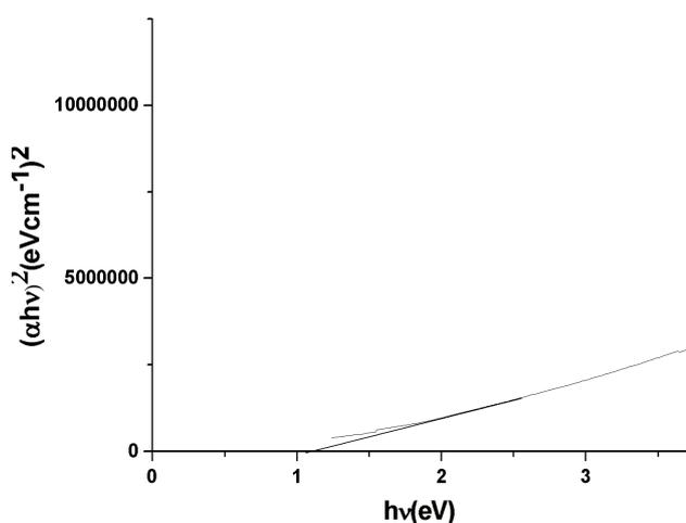
Fig. 13. Direct allowed transition energy gap of PANI(HCl).
