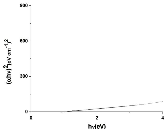
Fig. 15. Direct allowed transition energy gap of PANI(HCl)-MWNT(1:0.5) composite.
