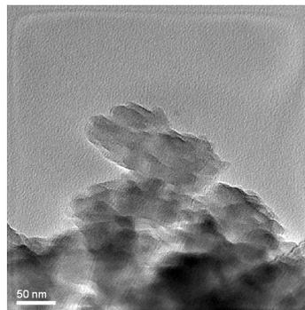
Fig. 4. TEM image of PANI(HCl)-MWNT(1:0.5) composite.
