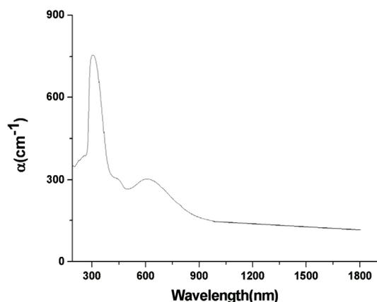
Fig. 6. Optical absorption spectrum of PANI(EB) cast from m-cresol.
