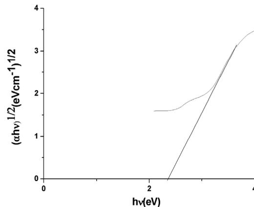
Fig. 12. Indirect allowed transition energy gap of PANI(EB) cast from m-cresol.
