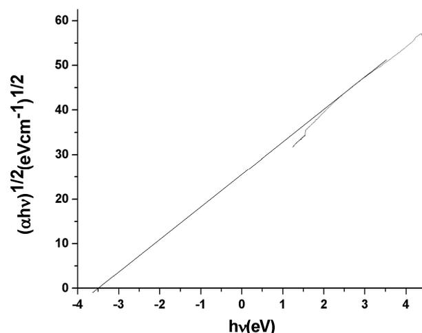
Fig. 16. Indirect allowed transition energy gap of PANI(HCl)-MWNT(1:0.5) composite.
