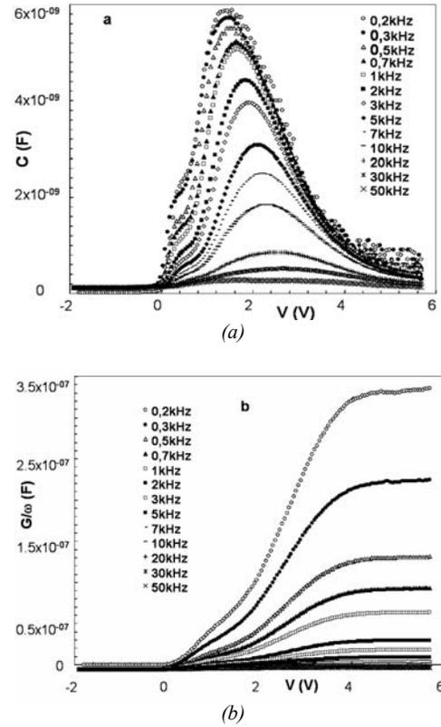
Fig. 1. The  $C$ - $V$ - $f$  and  $G/\omega$ - $V$ - $f$  characteristics of MIS structure, respectively, at room temperature.
