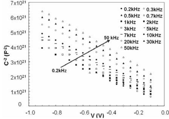
Fig. 2. The forward-bias  $C^{-2}-V$  characteristics of Al/SiO<sub>2</sub>/p-Si structure at room temperature.
