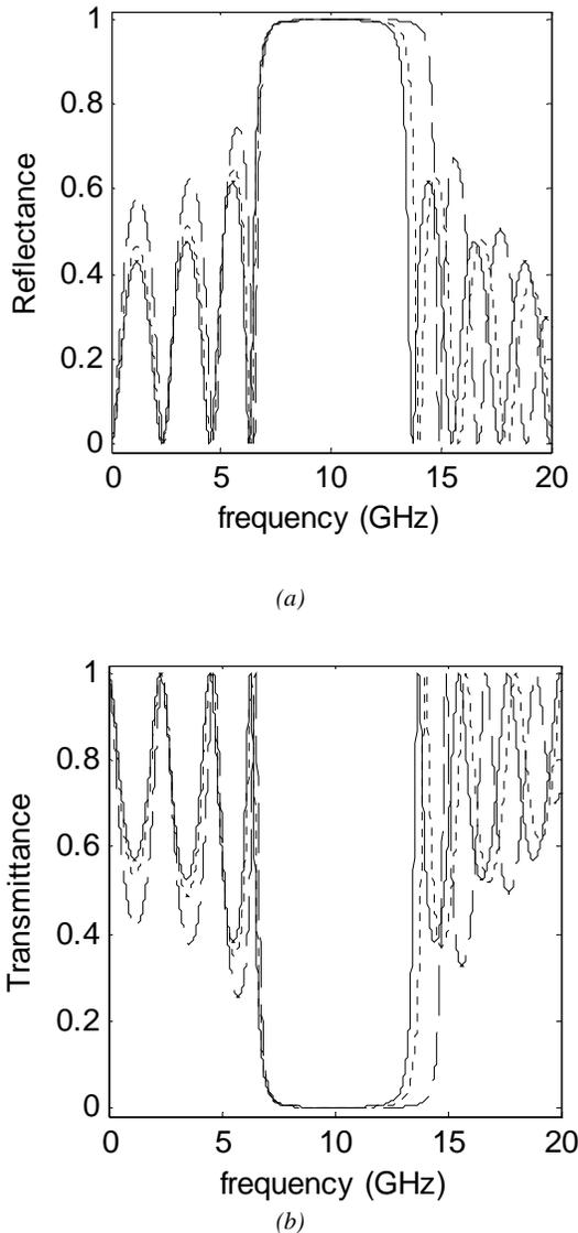
Fig. 1 Reflectance and transmittance for all dielectric layers as a function of the frequency for the incidence angles of  $0^\circ$ ,  $20^\circ$ , and  $40^\circ$ . Solid lines correspond to  $0^\circ$ , dotted lines to  $20^\circ$ , and dashed lines to  $40^\circ$ .
