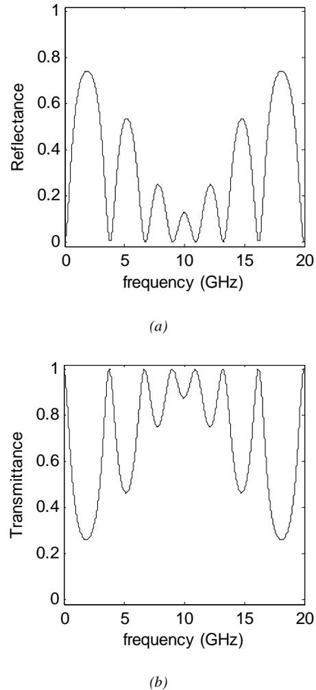
Fig. 4. Reflectance and transmittance for half wavelength long NRI and quarter wavelength long PRI layers versus the frequency.
