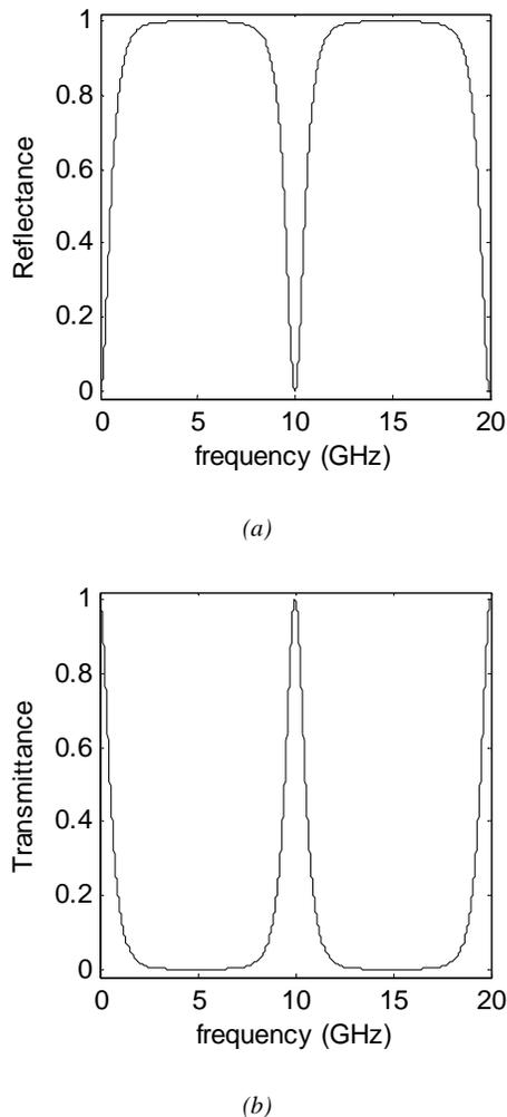
Fig. 3. Reflectance and transmittance for half wavelength long seven NRI and PRI layers against the frequency.
