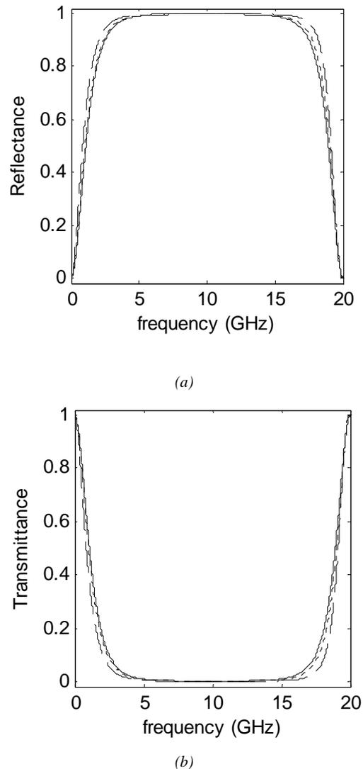
Fig. 2. Reflectance and transmittance for NRI and PRI layers versus frequency for the incidence angles of  $0^\circ$ ,  $20^\circ$ , and  $40^\circ$ . Solid lines correspond to  $0^\circ$ , dotted lines to  $20^\circ$ , and dashed lines to  $40^\circ$ .
