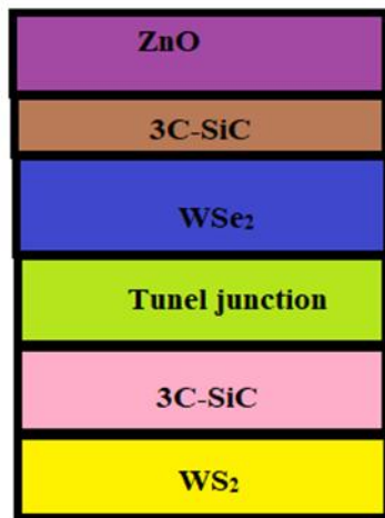
Fig. 1. Design of the cell WSe 2 /WS 2 (colour online)
