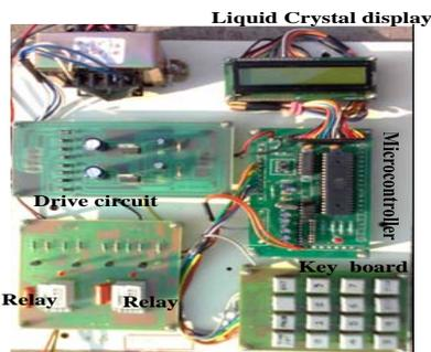
Fig. 3. Photograph of the microcontroller circuit.
