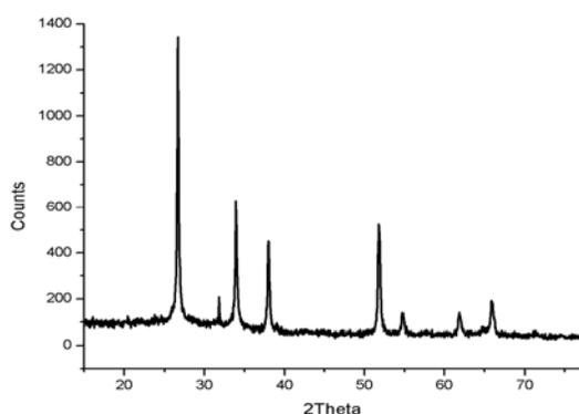
Fig. 7(b). XRD of SnO-F on glass substrate.
