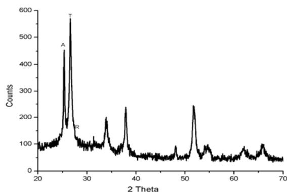
Fig. 7(c). XRD of SnO-F &  $\text{TiO}_2$  on glass substrate.
