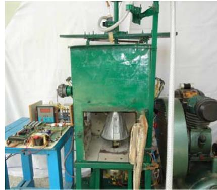
Fig. 4. Photograph of the microcontroller circuit & inclined substrate for spray pyrolysis set up.
