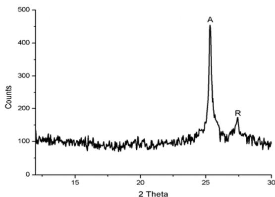
Fig. 7(a). XRD of  $\text{TiO}_2$  on glass substrate.
