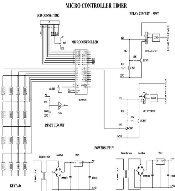
Fig. 2. The overall circuit diagram of the microcontroller circuit.
