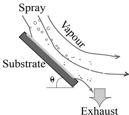
Fig. 6. Aerosol transport on an inclined substrate.
