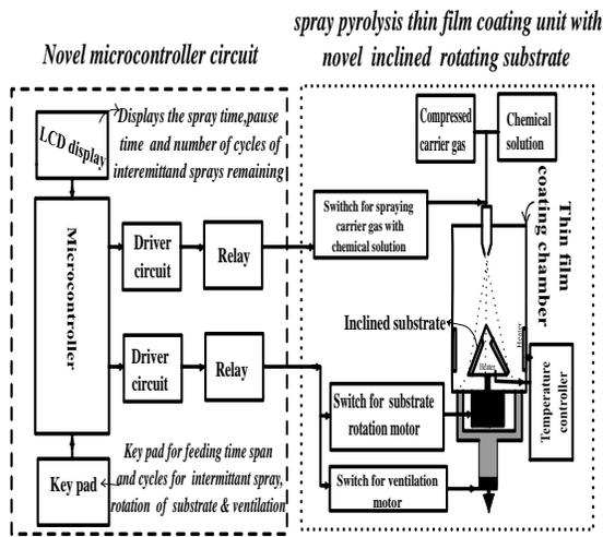
Fig. 1. Block diagram of the newly developed spray pyrolysis set up.
