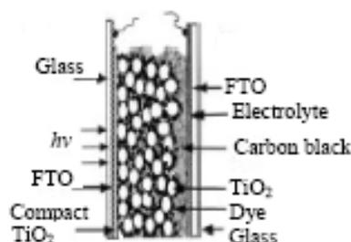
Fig. 10. Schematic diagram representing the DSSC layers (side view). The thickness of the thin film layers from right: 1 mm glass plate, 2.8  $\mu\text{m}$  FTO layer, 6  $\mu\text{m}$  sensitized nanoporous  $\text{TiO}_2$ , 100 nm compact anatase  $\text{TiO}_2$  layer, 2.8  $\mu\text{m}$  FTO layer, 1mm glass plate.
