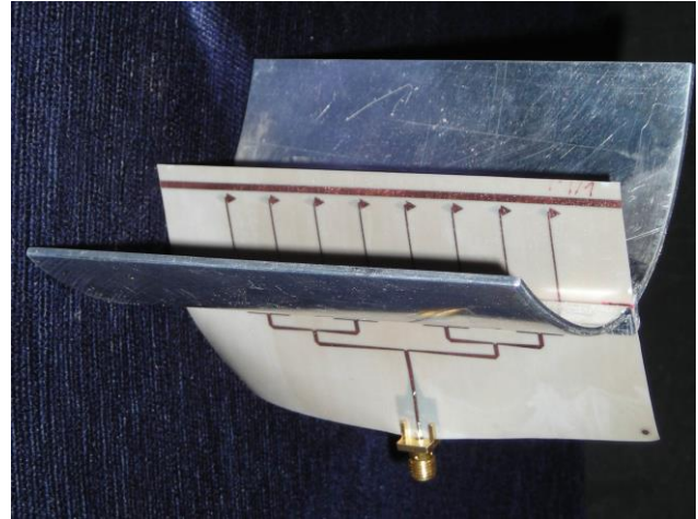
Fig. 10. Photograph of the realized antenna array with a subreflector in cylindrical-parabolic reflector.
