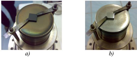
Fig. 5. Steel sample on the holder of the PLD device: a) before and b) after the alumina PLD deposition.
