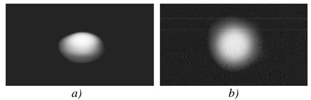
Fig. 2 a), b). Near-field image of the fundamental mode in a Er<sup>3+</sup>:Ti:LiNbO<sub>3</sub> Waveguide a) and single - mode optical fiber b).
