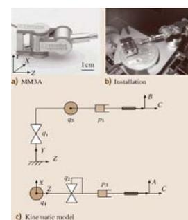
Fig. 2. Nanomanipulator (MM3A from Kleindiek) inside a SEM.
