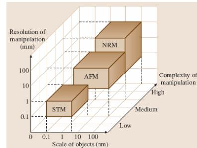
Fig. 1. Comparison of nanomanipulators.
