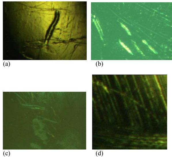
Fig. 5. Images obtained with the device Hexapod system for Micro - Movement F-206 - AFM. Images of cutting (a), scratches (b, d) and particle (c) on Co-Cr femoral head of a hip prosthesis (MEMS/NEMS Laboratory, INCDMTM).
