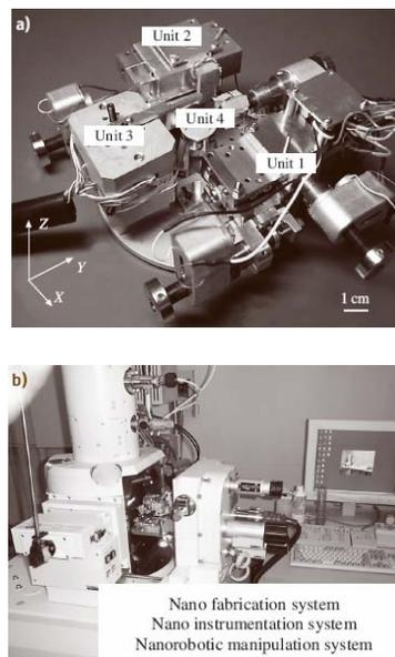
Fig. 3. a, b. Nanorobotic system. (a) Nanorobotic manipulators. (b) System set-up.
