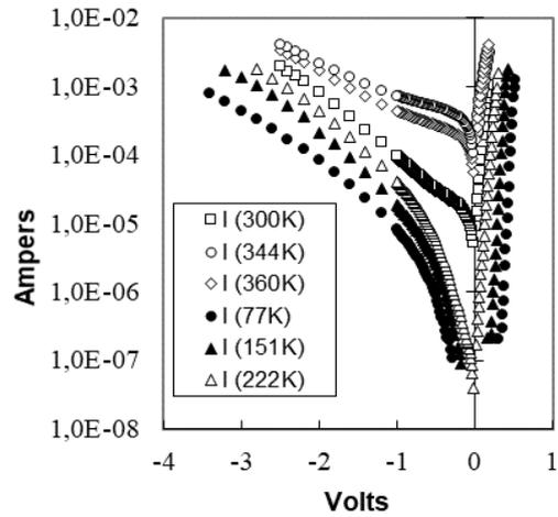
Fig. 1. Current-voltage characteristics of GaSb-GaInAsSb-GaSb heterojunctions at several temperatures
