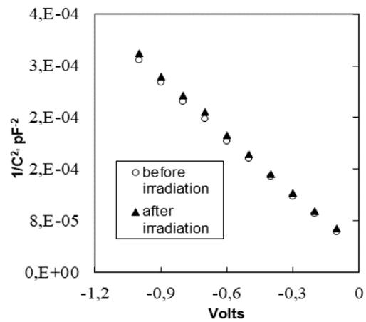
Fig. 4. Capacitance-voltage characteristics of the investigated GaSb-GaInAsSb-GaSb heterojunctions temperatures before and after <sup>60</sup>Co Gamma irradiation
