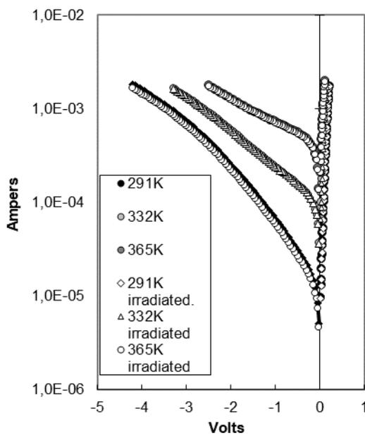
Fig. 3. Comparison of the current-voltage characteristics at high temperatures before and after <sup>60</sup>Co Gamma irradiation with photon energy of 6 MeV
