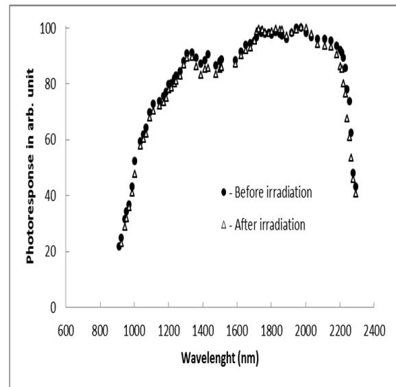
Fig. 5. Spectral distribution of photosensitivity for the GaSb- GaInAsSb-GaAlAsSb heterojunctions after <sup>60</sup>Co Gamma irradiation with photon energy of 6 MeV
