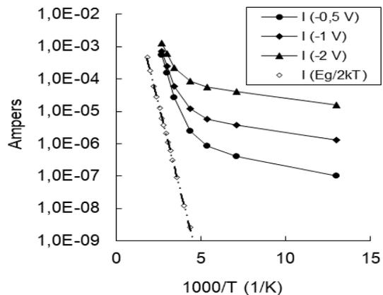
Fig. 2. The reverse current as a function of reciprocal temperature at different reverse applied bias
