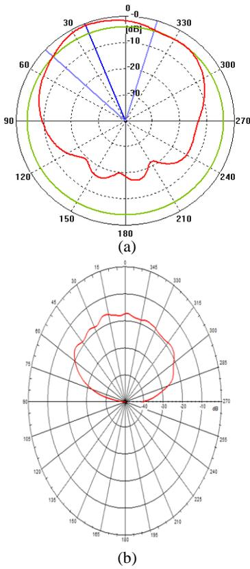
Fig. 7. (a) Simulated radiation pattern; (b) Measured radiation pattern for the broad beams at the Wilkinson Power Dividers output port 5.
