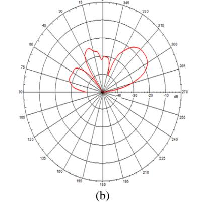
Fig. 5. (a) Simulated radiation pattern; (b) Measured radiation pattern for the narrow beams at the Butler matrix output port 3.
