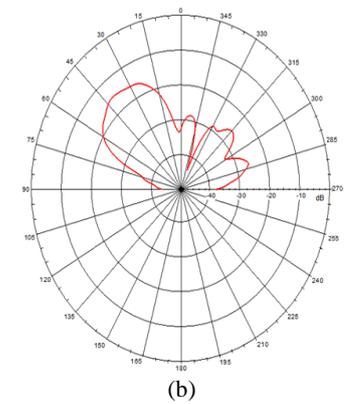
Fig. 4. (a) Simulated radiation pattern; (b) Measured radiation pattern for the narrow beams at the Butler matrix output port 2.
