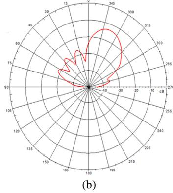
Fig. 3. (a) Simulated radiation pattern; (b) Measured radiation pattern for the narrow beams at the Butler matrix output port 1.
