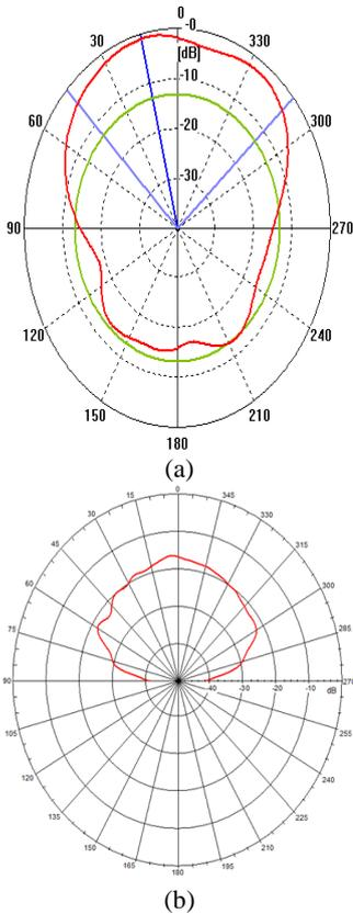
Fig. 8. (a) Simulated radiation pattern; (b) Measured radiation pattern for the broad beams at the Wilkinson Power Dividers output port 6.
