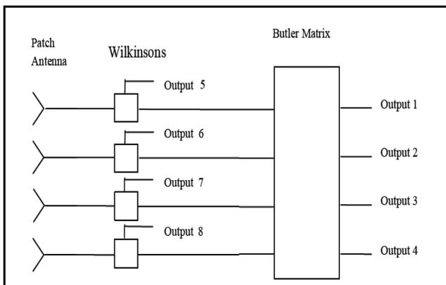
Fig. 1. Block diagram of dual beam antenna system.
