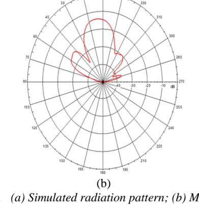
Fig. 6. (a) Simulated radiation pattern; (b) Measured radiation pattern for the narrow beams at the Butler matrix output port 4.
