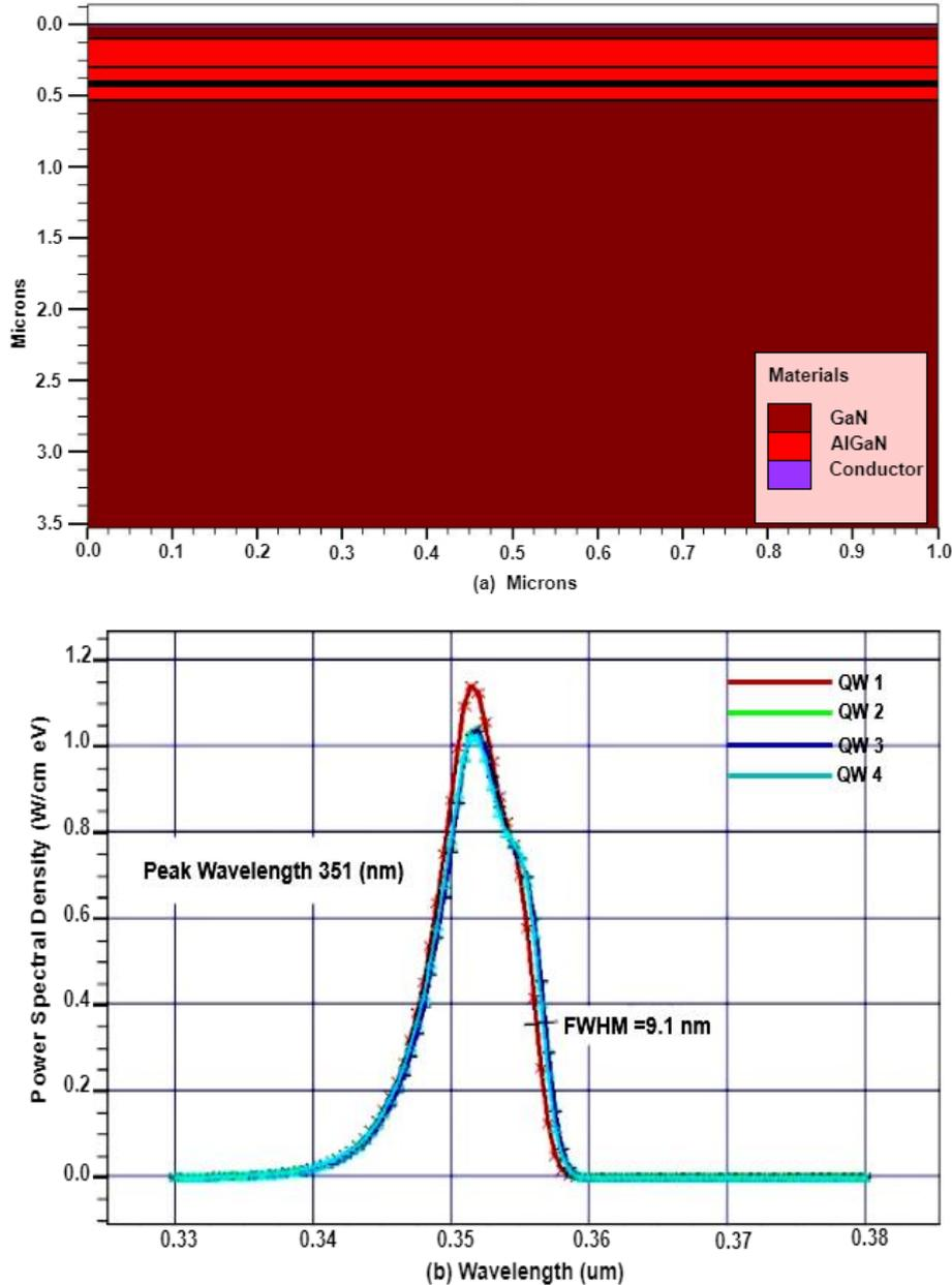
Fig. 2. (a) Simulation results of GaN MQW-LED (b) PSD vs wavelength curve (color online)
