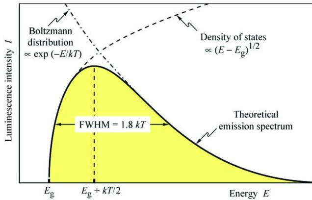
Fig. 1. Typical Emission Curve for LED [8]
