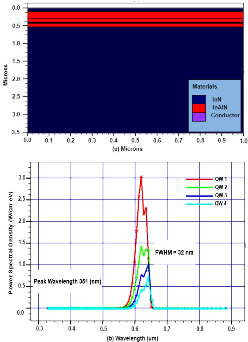
Fig. 3. (a) Simulation results of InN MQW LED (b) PSD vs wavelength curve (color online)
