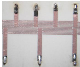
Fig. 7. Microscopic view of the metamaterial coupled structures
