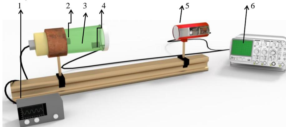
Fig. 7. Sketch of the experimental setup: 1-microwave generator power supply; 2- magnetron antenna; 3- cylindrical waveguide; 4-inductor; 5-cosmic rays detector; 6- oscilloscope
