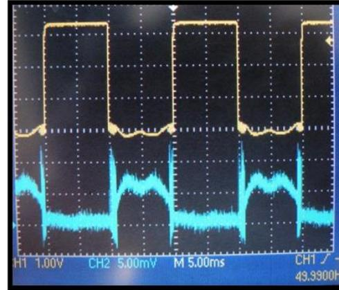
Fig. 6. Yellow oscillogram- supply voltage waveform of the magnetron. Blue oscillogram- the microwave field waveform inside of the cylindrical waveguide
