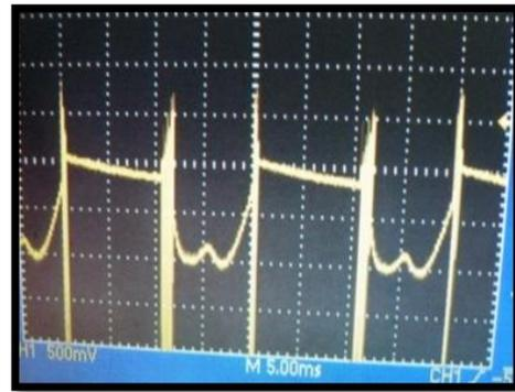
Fig. 9. The signal output of charge sensitive preamplifier with scintillator to  $0^\circ$
