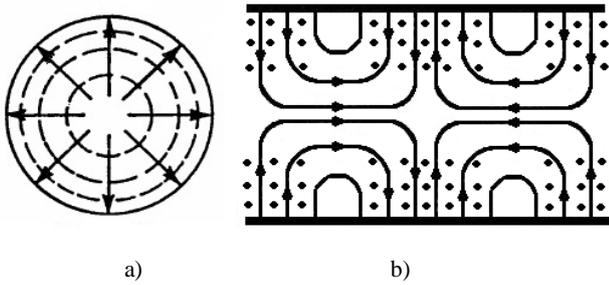
Fig. 5. Field distribution of  $TM_{01}$  mode in the cylindrical waveguide: a) Cross-Sectional view; b) Longitudinal view
