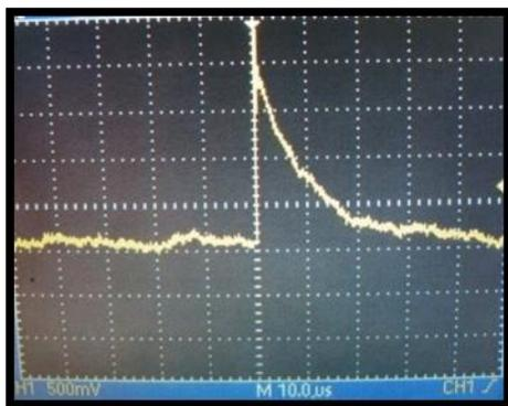
Fig. 3. Pulse shape of preamplifier
