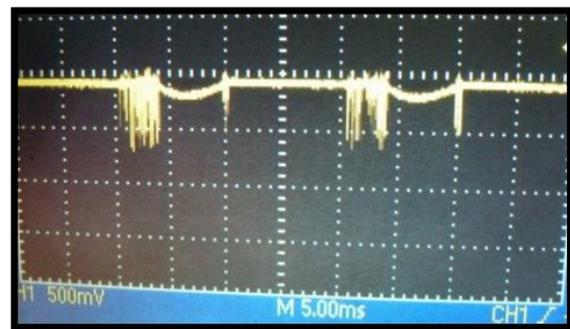
Fig. 11. The signal output of charge sensitive preamplifier without scintillator and positioned at  $0^\circ$
