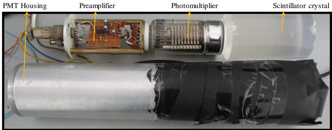
Fig. 1. Image of typical cosmic rays detector
