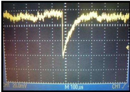
Fig. 2. Pulse shape of output PMT anode
