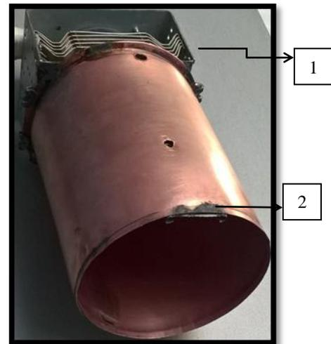
Fig. 4. Image of microwave generator: a) magnetron; b) cylindrical waveguide
