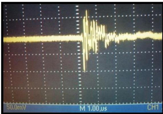
Fig. 8. PMT output signal with scintillator at  $0^\circ$
