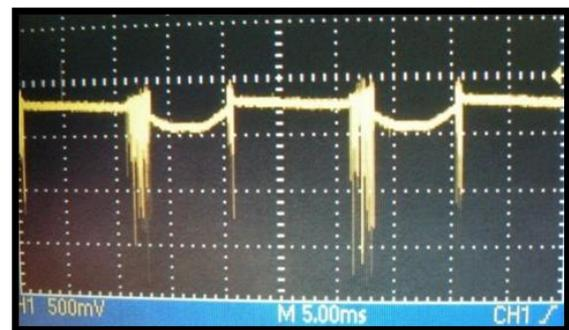
Fig. 10. The signal output of charge sensitive preamplifier with scintillator to  $90^\circ$
