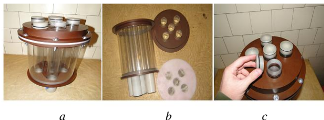
Fig. 1. View of the adsorption module for aniline: a - overview; b - components of the module; c - fixing the adsorbent material.
