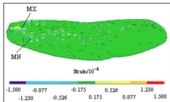
Fig. 11. The strain of the finite element model of a dragonfly forewing under the uniform load.
