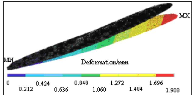
Fig. 9. The deformation of the finite element model of a dragonfly forewing under the uniform load.
